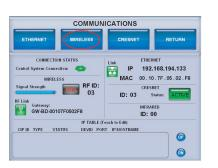
Before a TPS-6X can be used on a wireless network, it must first be acquired by a CEN(I)-ERFGW-POE Extended Range RF Wireless Gateway (sold separately).
