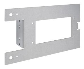
The Crestron® TSW-UMB-70-PMK preconstruction mounting kit provides a complete preconstruction mounting solution for TSW-570, TSW-770, TSW-1070, TSS-770, and TSS-1070 series touch screens. The TSW-UMB-70-PMK is designed to be used along with the TSW-UMB-70 universal mounting bracket and permits fastening to the left or right-hand stud of a framed wall prior to installing drywall.
