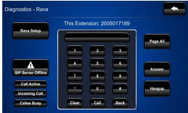
The **Diagnostics - Rava** screen provides controls for testing the use of Crestron's Rava SIP Intercom with the FT-TS600. It can be used to test projects and settings. If the intercom works but the project does not, there is an issue with the project; if the intercom does not work, there is an issue with the settings.
