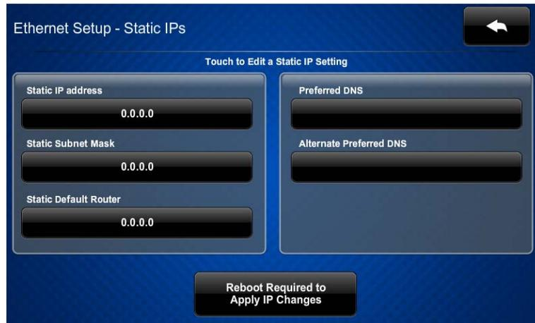
To edit the static IP address, static subnet mask, static default router, preferred DNS, or alternate preferred DNS, tap its corresponding field. The **Edit IP Address** screen opens.
