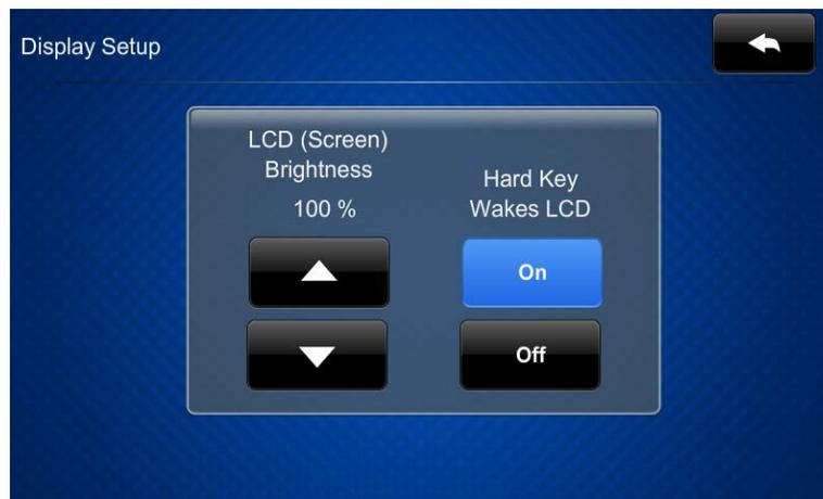
The **Display Setup** screen provides controls for the screen's LCD brightness and **On** and **Off** controls for using a hard key to wake the LCD.
