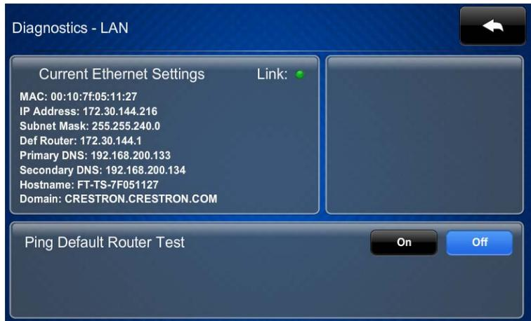
The **Diagnostics – LAN** screen displays current Ethernet settings and contains a link indicator to show the status of the Ethernet connection. A **Ping Default Router Test** control is also provided.
