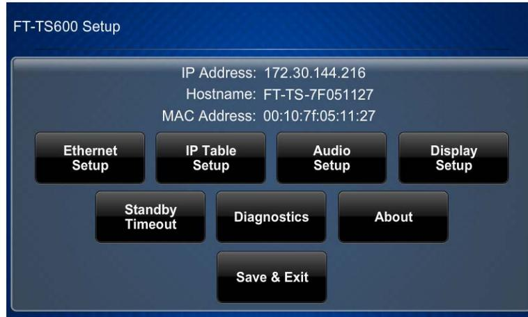
The FT-TS600 Setup screen is comprised of buttons for Ethernet setup, IP table setup, audio setup, display setup, standby timeout, and diagnostics. In addition, there is an **About** button that provides information about the touch screen and a **Save & Exit** button. The functions of each are detailed in the sections that follow.
