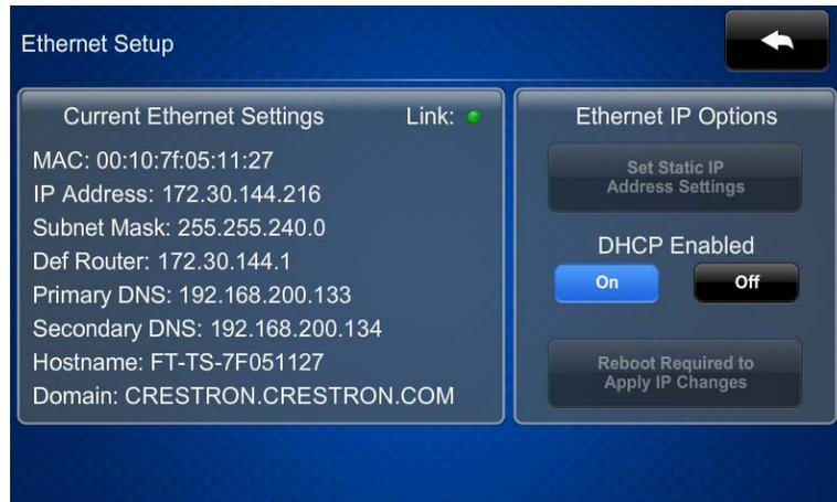
The **Ethernet Setup** screen displays the touch screen's Mac and IP addresses, subnet mask, default router, primary DNS, secondary DNS, hostname, and domain. This screen also contains a link indicator to show the status of the Ethernet connection.
