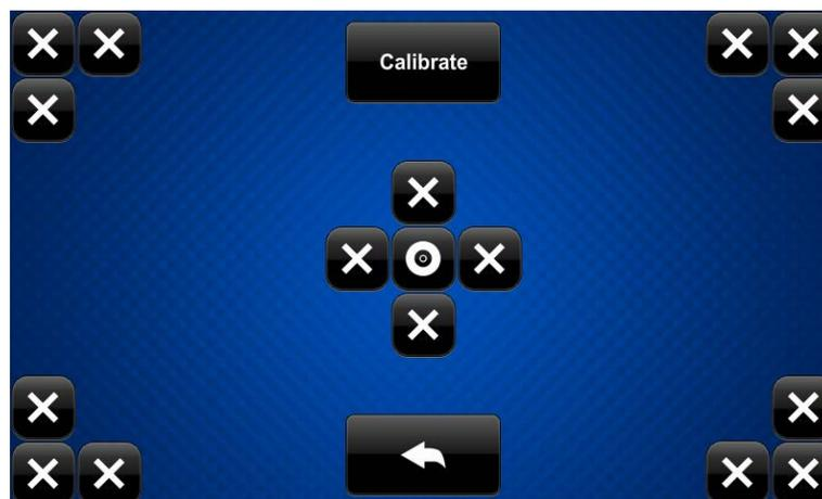
The touch test screen can be used to test the function of the screen. When a location button (the **X** buttons or the **O** button) is tapped, its indicator on the screen lights. This screen also contains a **Calibrate** button to initiate touch screen calibration.
