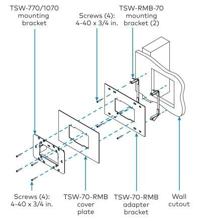
5. Attach the touch screen to the TSW-770/1070 mounting bracket to complete the installation.
