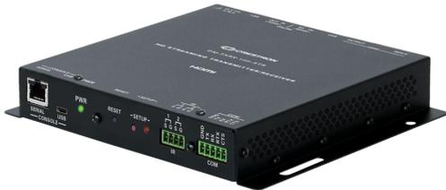
The DM-TXRX-100-STR is a compact H.264 streaming encoder and decoder designed to enable distribution of high-definition AV signals over an IP network. It is configurable as either a transmitter or receiver and is a perfect complement to any DigitalMedia switcher with one or more streaming inputs or outputs. The DM-TXRX-100-STR can also be used to add streaming capability to other switchers and devices.
