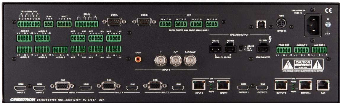
The DMPS3-300-C integrates the control system, multimedia matrix switcher, mic mixer, audio DSP, amplifier, and DigitalMedia distribution center all into a single 3-space rack-mountable package. The DMPS3-300-C affords substantial signal-routing flexibility and high-performance signal processing without the need for separate components. The preloaded DMPS3 .AV Framework software enables customized configuration and control without programming.
