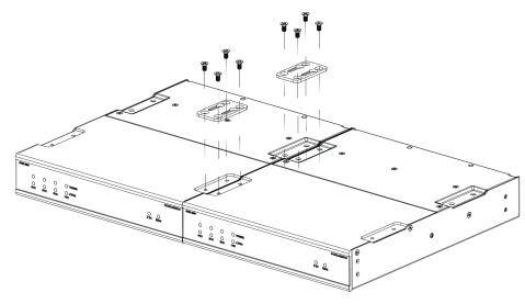
3. Use a wrench or M5.5 socket to remove the nuts from the rack ears.
