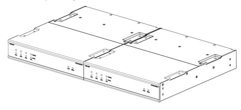
2. Use a Phillips screwdriver to gang the amplifiers together with two of the joining plates and the eight  $8-32 \times 5/16$  in. screws.
