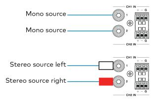
NOTE: RCA and terminal block inputs with the same channel number are summed.
