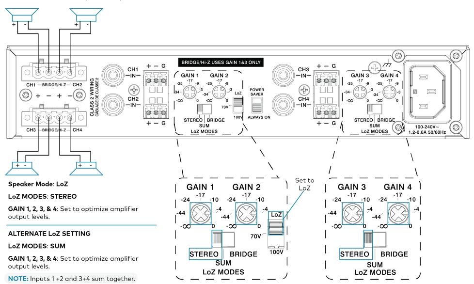
2 Channel x 150 W Bridged Stereo Output (Low Impedance)
