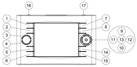
**NOTE:** Join numbers 16 and 17 are fixed for the two "trigger" keys, the top-mounted pushbuttons on the TPS-6X. The left trigger key toggles power when the unit is undocked and initiates *Sleep* mode when docked. In addition, when held for five seconds, it initiates a touchpanel reset. The right trigger key toggles screen brightness, unless it is disabled with the on-screen button in the BACKLIGHT SETUP menu (refer to "BACKLIGHT" which starts on page 30).
