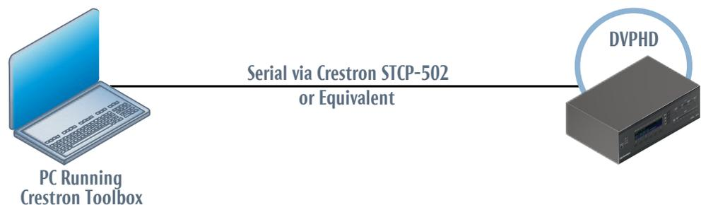
The **RS-232** port on the DVPHD connects to the serial port on the PC via a serial cable (Crestron STCP-502 or equivalent):
