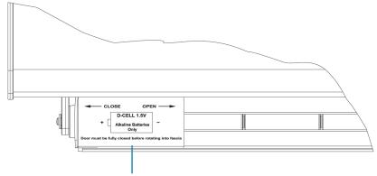
Slide battery door closed after the batteries are installed. The door clicks into place.
