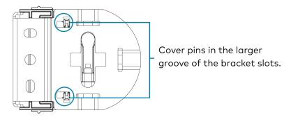
2. Move the cover so that the pins slide to the thinner groove of the bracket slots and the cover clicks into place.
