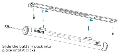
3. Connect the battery-pack cable to the motor.
