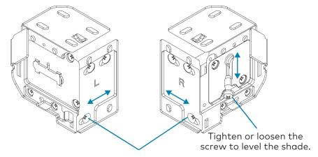
Loosen the screws, adjust the shade so that it is centered in the opening, and then tighten the screws to lock the shade into place.
