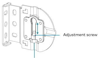
To level the shade, use a 1.5 mm allen key (not included) to tighten or loosen the screw.
