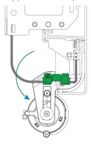
3. Slide the battery door into the **OPEN** position.
