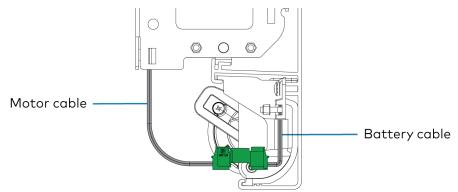
To disconnect battery assembly from motor, disconnect the connector on the motor cable from the connector on the battery cable.
