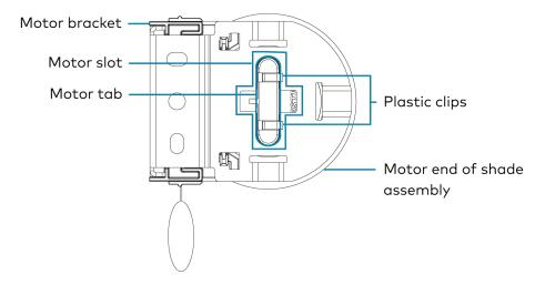
Maneuver the motor end of the shade assembly into the bracket slot. Plastic clips lock the motor into the motor bracket when the motor is fully inserted. Pull the motor end gently away from the motor bracket to ensure that the motor is securely locked into place.
