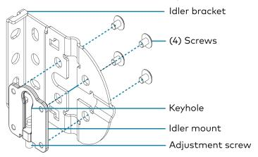
Remove the screws and separate the idler mount from the idler bracket.
