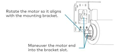
4. Push the tab on the motor end of the shade assembly into the motor slot of the motor bracket. When the shade is properly seated, the two plastic clips spring down to secure the motor to the motor bracket. Make sure that the shade is properly mounted before letting go.
