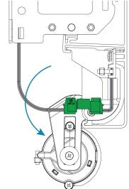
Rotate battery pack to original position. Battery pack clicks into position.
