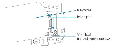
2. Raise and align the motor end of the roller shade assembly to the motor bracket.
