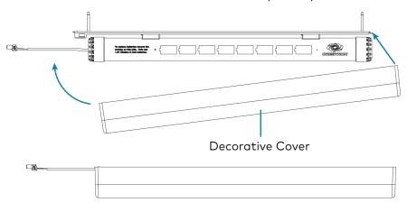
To remove the decorative cover, squeeze the decorative cover near the end where the motor exits and then pull the cover away from the mounting bracket.
