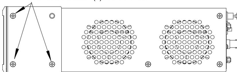
Right side view of C2N-DVP4DI with optional rack mounting ears installed.
