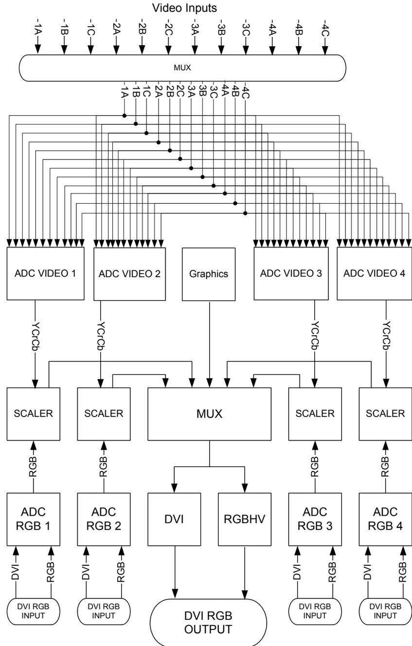
For example: Selecting video 1a causes the C2N-DVP4DI to choose scaler 1. Selecting video 1b causes the C2N-DVP4DI to select scaler 2. If you then select RGB1, the C2N-DVP4DI moves video 1a to scaler 3 and then brings up RGB 1.
