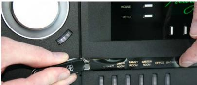
4. Continue sliding the screwdriver until the entire top of the label strip is visible. Remove the label strip by pulling the top of the label strip up from the Adagio component as shown below.
