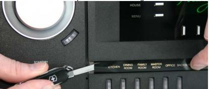
Continue sliding the screwdriver behind the label strip until the top of the label strip slides out as shown below.
