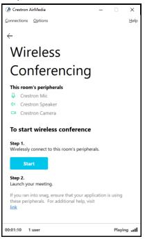
Pressing the blue **Start** button on the presentation screen or peripheral information screen will connect the computer to those peripherals. This will allow their use in most meeting room applications. On the room display, icons for each connected device type (camera and/or microphone) will appear.
