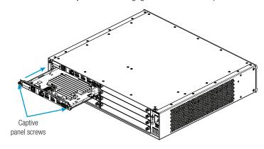
Finger-tighten the two captive panel screws to secure the card—do not overtighten the screws.
