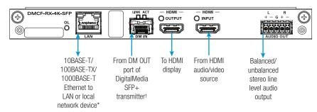
\*To connect to the LAN, use either the LAN port of the DMCF-RX-4K-SFP receiver or the LAN port of the companion transmitter (DMCF-TX-4K-SFP or DMF-TX-4K-SFP)—do not connect the receiver and transmitter LAN ports to the LAN simultaneously.
