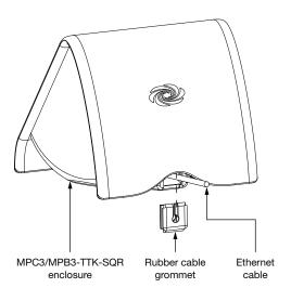
Complete the MPC3-201 installation and configuration as described in the MPC3-201 DO Guide (Doc. 7876).
