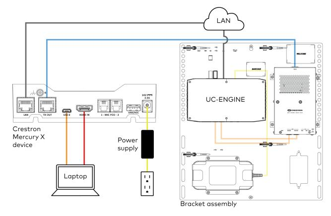
3. Connect the display devices and camera to components on the bracket assembly as shown below.
