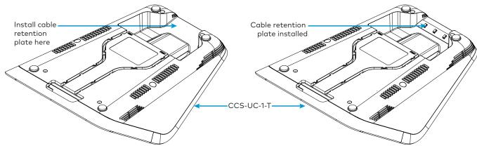
NOTE: Before securing cables, ensure the cable retention plate is firmly attached.
