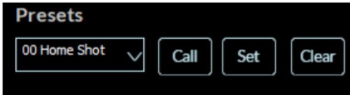
Open the **Presets** drop-down menu by selecting the down arrow to display all camera presets. Select the desired preset to set it as the active preset. The **Call**, **Set**, and **Clear** controls will be applied to the active preset.
