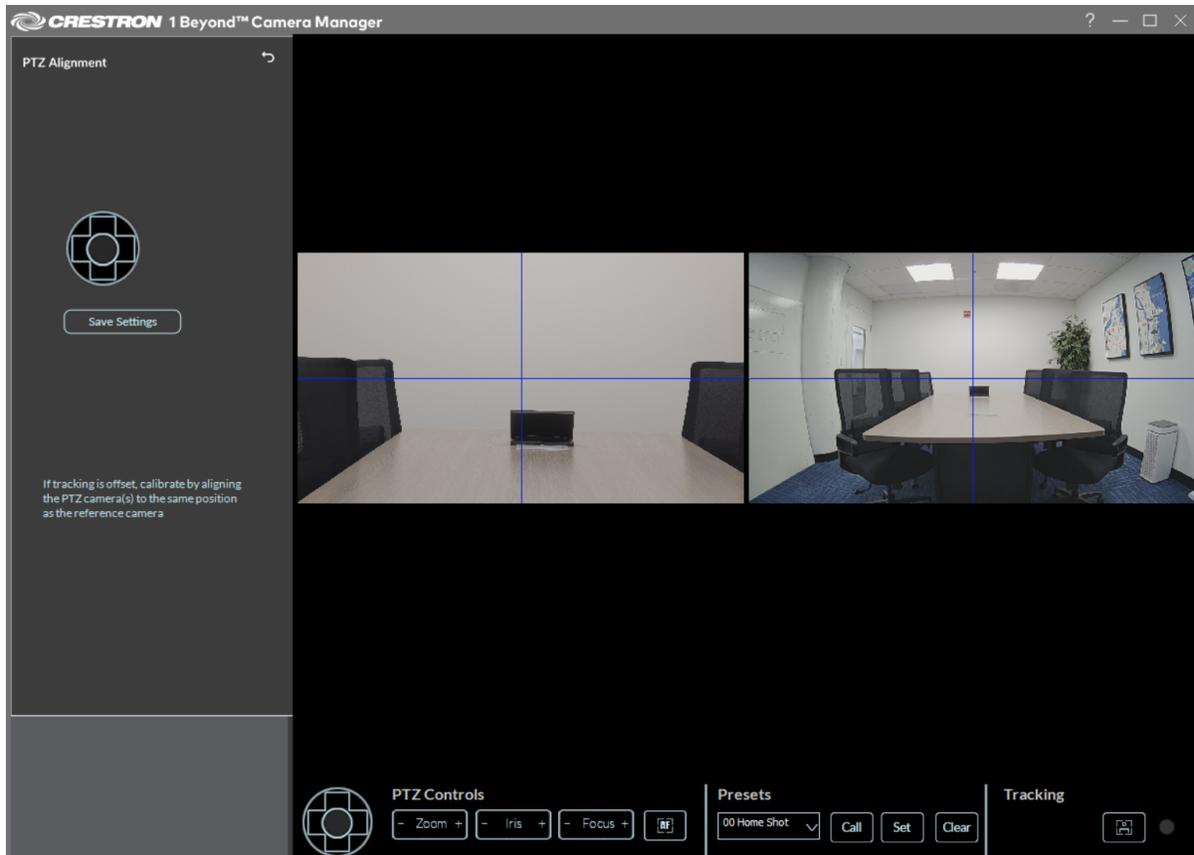
3. Use the PTZ lens controls in the **Settings** panel to move the PTZ video feed's blue crosshair into the same position as the wide-angle feed's crosshair. For best results, place an object that can be seen in both camera feeds as a point of reference for the blue crosshairs.
