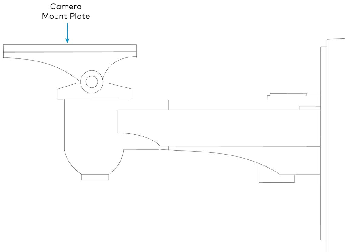
9. Use a 4 mm Allen Key wrench to loosen the hinge bolt on the side of the camera mount.
