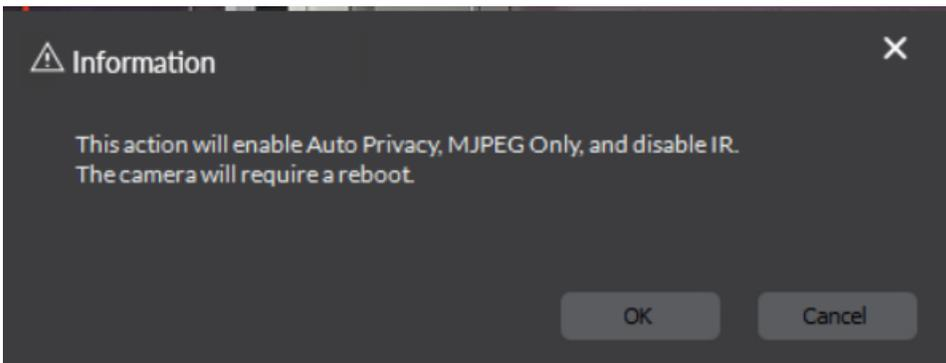
6. Select the **OK** button in the Information screen. The camera now optimizes its settings for Multi-Camera Switching (Auto Privacy enabled, MJPEG Only mode enabled, and disable the IR receiver).
