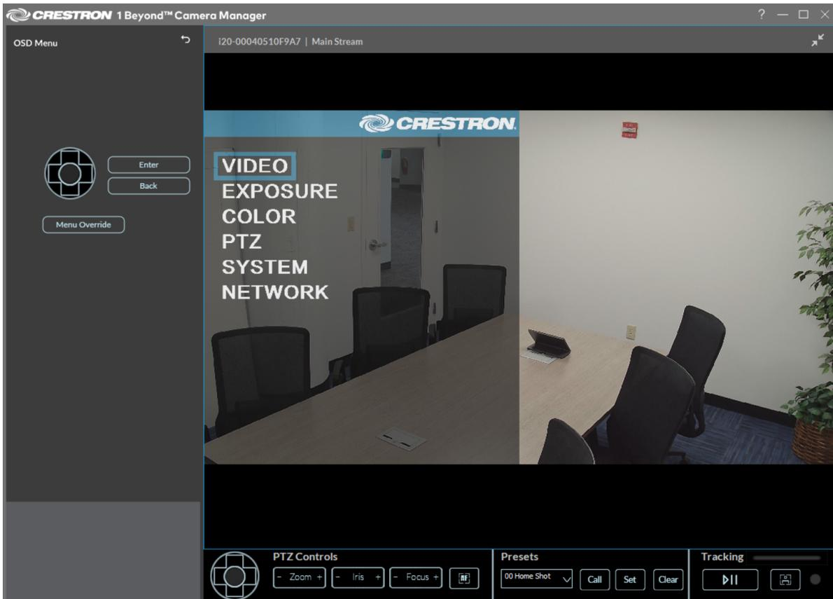
**TIP:** Alternatively, the OSD menu can be accessed with the [IV-CAMA-REMOTE](#) Crestron 1 Beyond IR Camera Remote. To access the OSD menu with the IR camera remote, press **Menu** on the remote.
