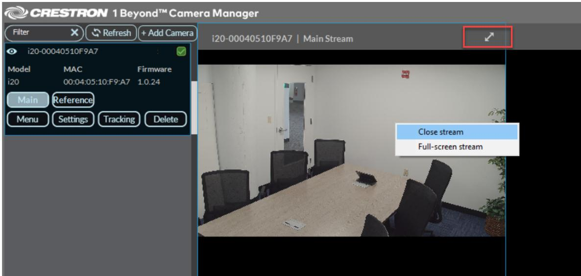
Alternatively, right click the desired video feed and select **Full-Screen Stream** to enter full screen borderless mode, hiding the user interface. Right click and select **Close Stream** to exit the full screen borderless mode.
