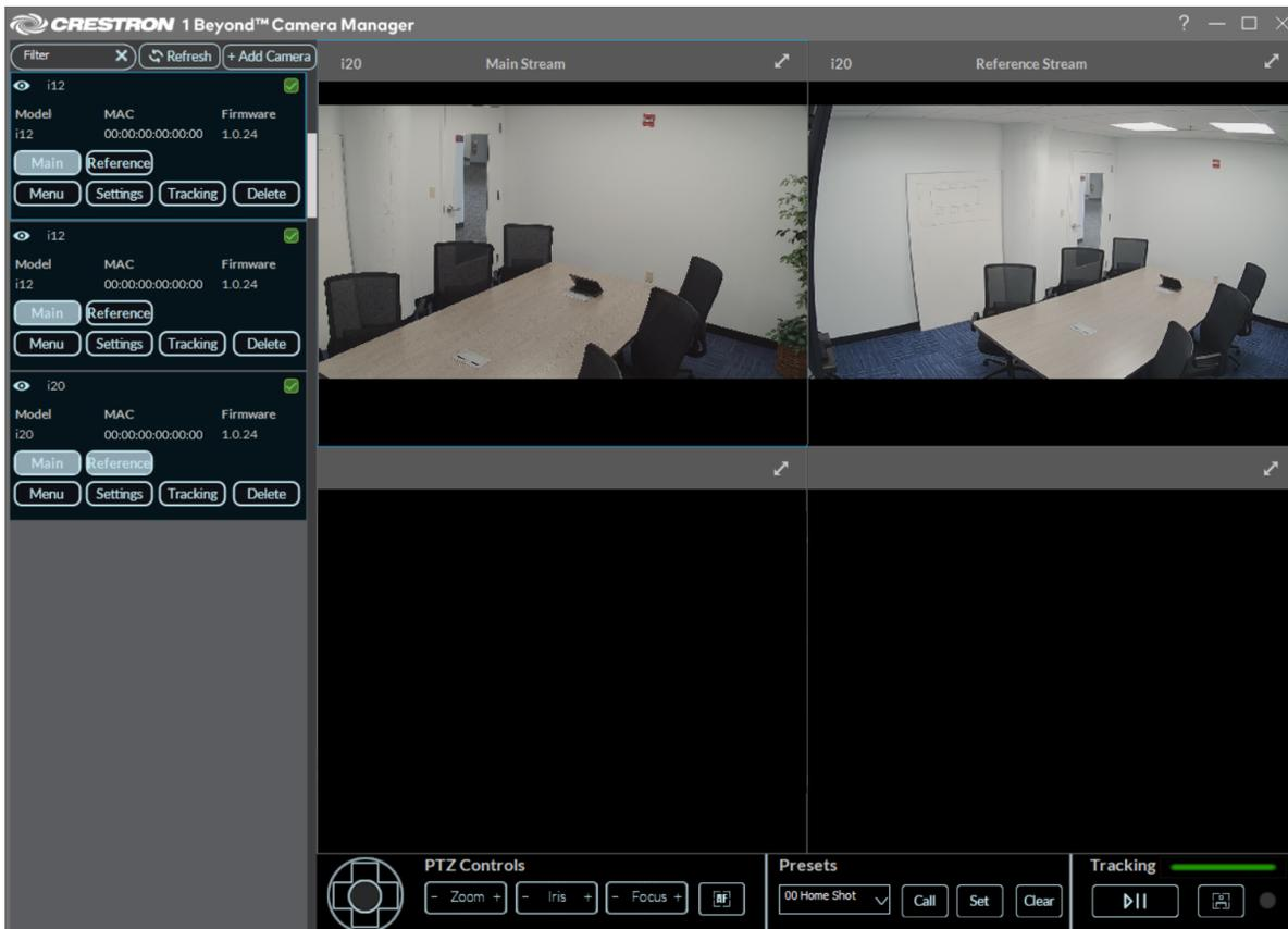
**NOTE:** If four camera feeds are displayed in the quad view, adding a new feed from the camera menu will replace the last added feed. To control the camera feed that is replaced, left click on the feed in the quad view before selecting a new feed
