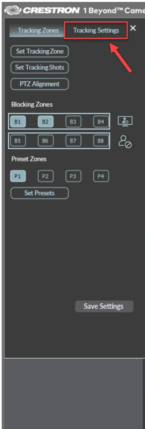
The **Tracking Settings** menu is displayed. The **Multi-Cam Tracking** settings are located at the bottom of the **Tracking Settings** menu.
