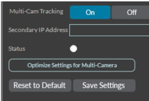
4. In the **Secondary IP Address** text field, enter the IP address of the Presenter Tracking camera (IV-CAM-I12 camera set to Presenter Tracking mode or an IV-CAM-I20 camera). For more information on setting an IP address for a camera, refer to [Set a Static IP Address on page 118](#).
