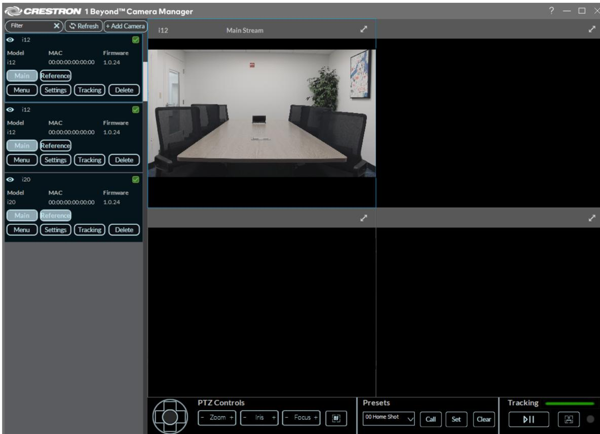
**NOTE:** If four camera feeds are displayed in the quad view, adding a new feed from the camera menu will replace the last added feed. To control the camera feed that is replaced, left click on the feed in the quad view before selecting a new feed.
