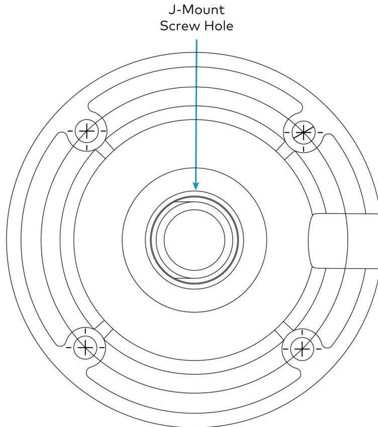
8. Use a Phillips® screwdriver to loosen the 2 x 1-1/2 in. screw near the bend on the J-Mount. Then, pull or retract the J-Mount to the desired length. Ensure that the 2 x 1-1/2 in. screw is retightened before proceeding.
