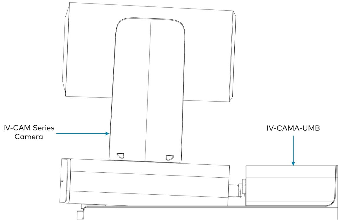
14. Tighten the two included M2.5 x 12 mm hand screws into the rear standoff holes on the camera.
