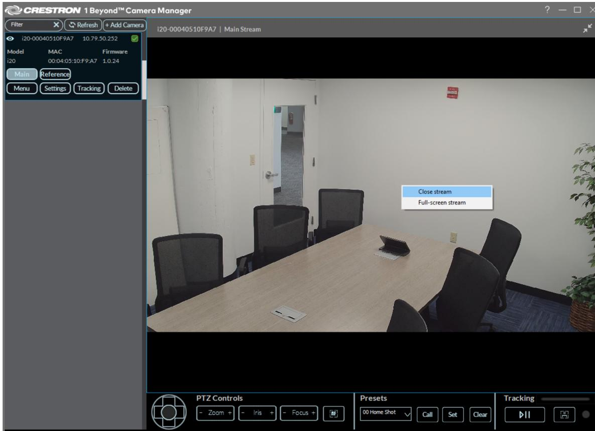
Alternatively, selecting the **Main** or **Reference** buttons closes the respective camera's video feed.
