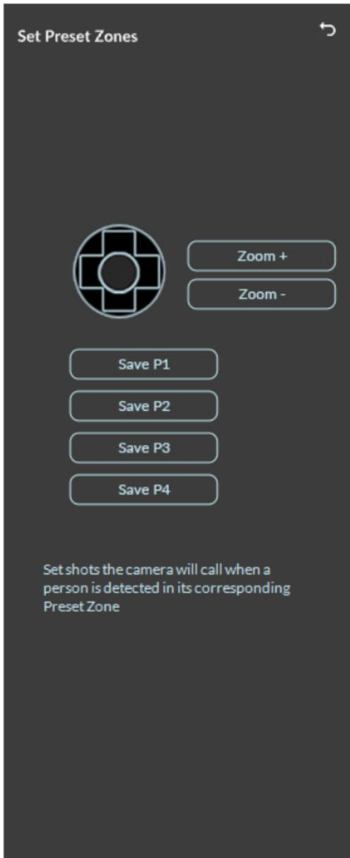
5. Use the navigation pad to pan and tilt the PTZ camera. The left and right buttons pan the camera, and the up and down buttons tilt the camera.
