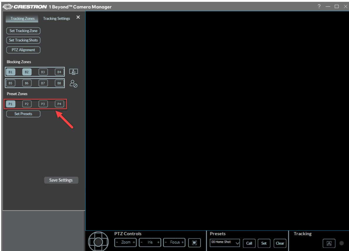
2. Press and hold the cursor over the location in the video frame where the **Preset Zone** should begin. Then, drag the cursor to draw the **Preset Zone**.
