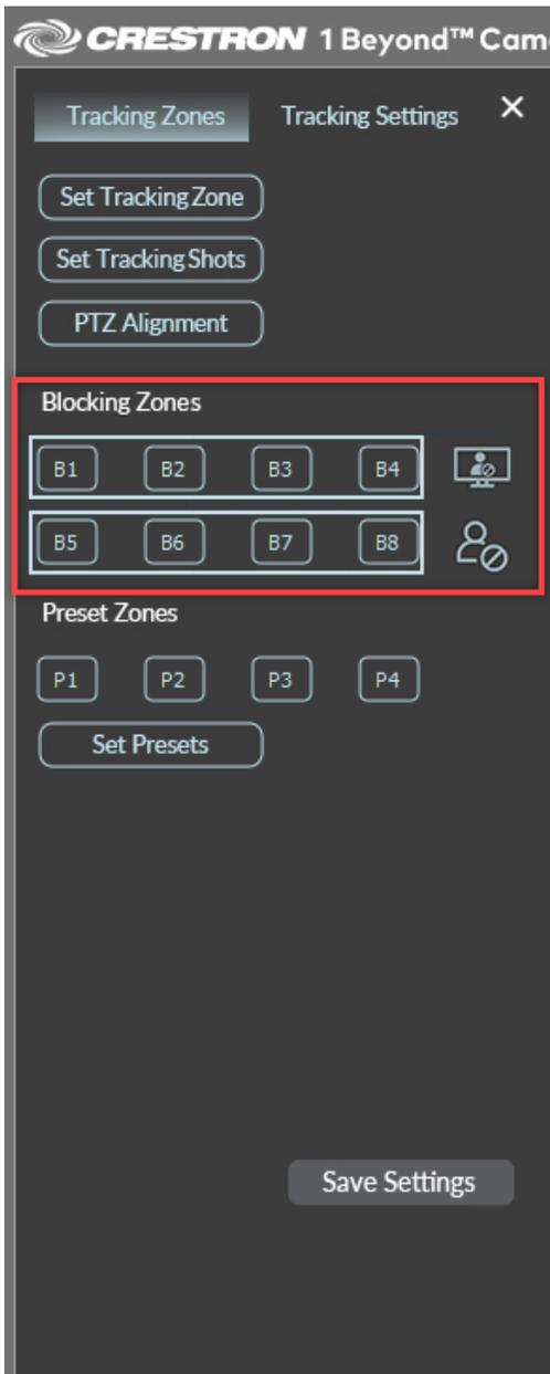
**Blocking Zones B1 through B4** are for blocking displays, windows, and projection screens.
