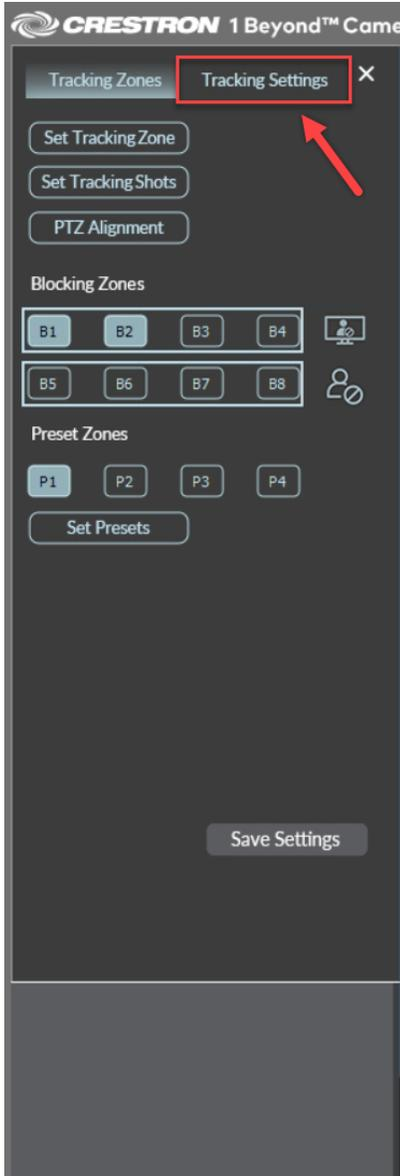
**NOTE:** The **Tracking Settings** menu contains different settings depending on whether an i12 or i20 camera is being configured. Additionally, if the i12 camera is in group framing mode, it contains different settings. For more information on changing the camera mode, refer to [Change the Camera Mode \(IV-CAM-I12/20 Only\) on page 125](#).
