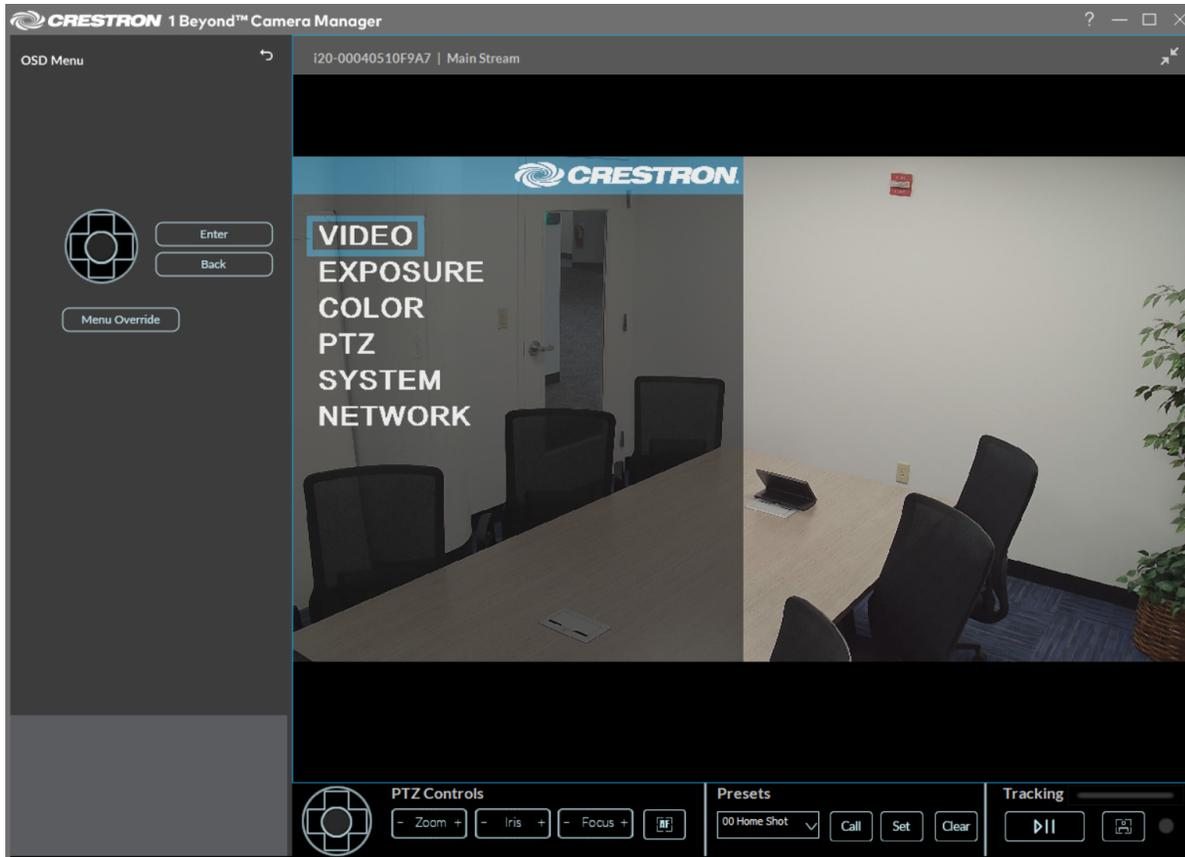
Alternatively, the OSD menu can be accessed with the [IV-CAMA-REMOTE](#) Crestron 1 Beyond IR Camera Remote. To access the OSD menu with the IR camera remote, press **Menu** on the remote.
