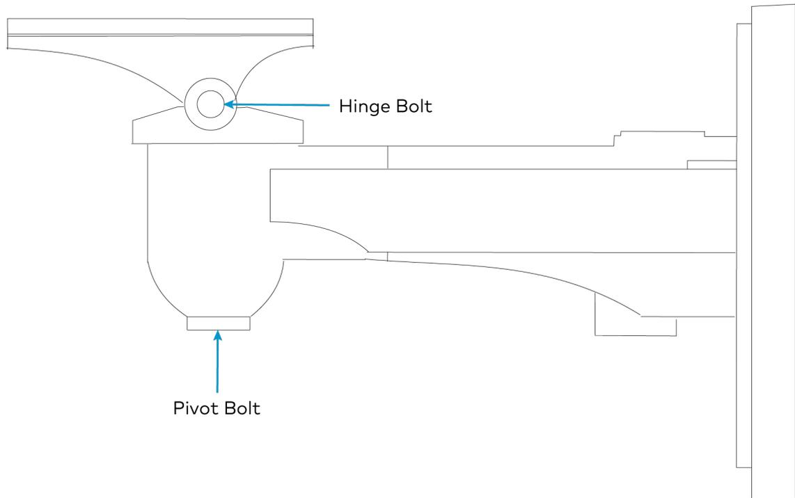
10. Tilt the camera mount plate to achieve the desired camera tilt. For information on tilt angles for cameras, refer to [Mounting Measurements on page 68](#)
