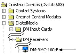
The system tree of the control system displays the DM-RMC-100-F in the appropriate slot with a default IP ID as shown in the following illustrations. In the first example, the DM-RMC-100-F is used with the DMCO-11 output card in a DM-MD8X8 switcher (both sold separately). In the second example, the DM-RMC-100-F is used with the C2ENET-2 card (sold separately) in an Ethernet slot on the control system.
