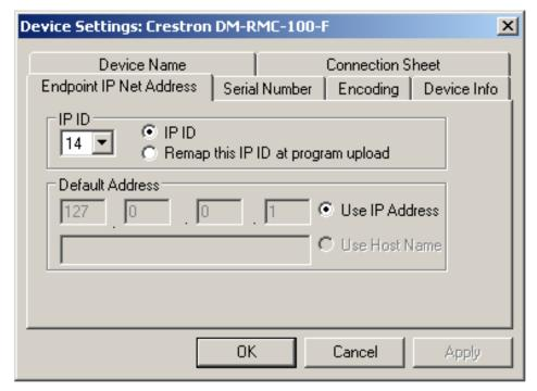
**NOTE:** The ID code specified in the SIMPL Windows program must match the IP ID of each unit. Refer to "Identity Code" which starts on page 17.
