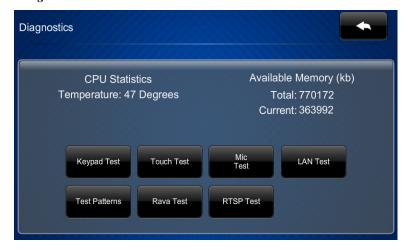
The "Diagnostics" menu displays the CPU temperature, *Available Memory* and contains controls to run a **Keypad Test**, **Touch Test**, **Mic Test**, **LAN Test**, **Rava Test**, and **RTSP Test**. In addition is a control to open various test pattern screens. These are explained in the paragraphs that follow.
