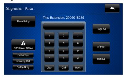
The "Diagnostics - Rava" menu provides controls for testing the use of Crestron's Rava<sup>TM</sup> SIP Intercom with the TSS-752. They can be used to test projects and settings. If the intercom works but the project does not, there is an issue with the project; if the intercom does not work, there is an issue with the settings.
