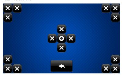
The touch test screen can be used to test the function of the screen. When a location button (the "x" buttons or the "o" button) is touched, its indication on the screen lights.
