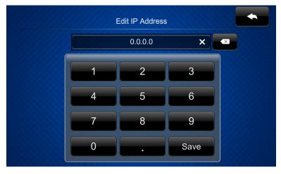
Use the keypad to make the new entry. Touch the "x" in the text field to clear any previous entry. Touch to delete the last digit. Touch **Save** to save a new entry or to return to the "Ethernet Setup – Static IPs" screen.
