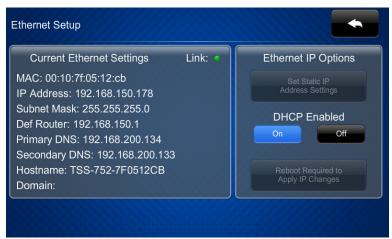
The "Ethernet Setup" menu displays the touch screen's MAC address and IP Address, Subnet Mask, Def Router, Primary DNS, Secondary DNS, Hostname and Domain. There are controls for turning DHCP On or Off as well as a Set Static IP Address Settings button, which provides access to controls which allow editing of these settings. This screen also contains a Link indicator to show the status of the Ethernet connection.
