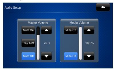
The "Audio Setup" screen provides controls for muting (or unmuting) the audio, adjusting level for both *Master Volume* and *Media Volume*, as well as a control for playing a test .wav file. The *Media Volume* controls adjust H.264 streaming media level in relation to the *Master Volume* controls.
