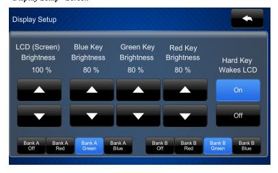
The "Display Setup" screen provides controls for LCD (Screen) Brightness, Blue Key Brightness, Green Key Brightness, Red Key Brightness, and **On** and **Off** controls for Hard Key Wakes LCD. In addition there are **Off**, **Red**, **Green**, and **Blue** controls for each bank of LEDs.
