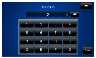
Use the keypad to make the new entry. Touch the "x" in the text field to clear any previous entry. Touch to delete the last digit. Touch **Save** to save a new entry or to return to the "Ethernet Setup – Edit IP Table Entry" screen.
