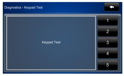
The "Diagnostics - Keypad" screen can be used to test the function of the hard key push buttons. When a button is pressed, its corresponding indication on the screen lights.
