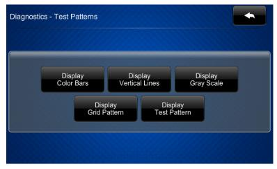
The "Diagnostics - Test Patterns" screen contains buttons for selecting the different available test patterns: **Display Color Bars**, **Display Vertical Lines**, **Display Gray Scale**, **Display Grid Pattern** and **Display Test Pattern**.
