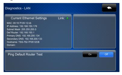
The "Diagnostics – LAN" screen displays the touch screen's *MAC* address and *IP Address*, *Subnet Mask*, *Def Router*, *Primary DNS*, *Secondary DNS*, *Hostname* and *Domain*. This screen also contains a *Link* indicator to show the status of the Ethernet connection and controls to test the connection to the default router.
