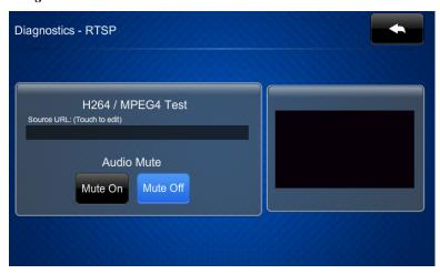
The "Diagnostics – RTSP" screen tests whether Real Time Streaming Protocol is functioning on the TSS-752. Touch the area below *Source URL: (Touch to edit)* to open the on-screen keyboard. Enter the URL for an H.264 or MPEG4 video and touch **Save**. The video is displayed on the right side of the "Diagnostics – RTSP" screen.
