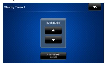
The "Standby Timeout" menu provides controls to adjust standby timeout from 0 to 120 minutes. There is also a Screen Saver Options button which opens the "Standby – Screen Saver" screen.
