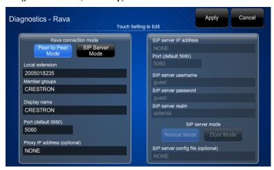
This screen provides controls to switch between **Peer to Peer Mode** and **SIP Server Mode**, and when in the latter, controls to switch between **Normal Mode** and **Door Mode**. Touching the other fields on the screen opens the on-screen keyboard or onscreen numeric keypad, as appropriate.
