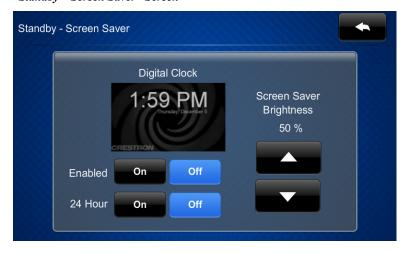
The "Standby – Screen Saver" screen provides controls to turn the *Clock Screen Saver* **On** and **Off** as well as controls to display the time in a *24 Hour* format and to adjust the *Screen Saver Brightness*.
