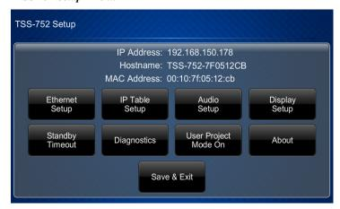
The "TSS-752 Setup menu" is comprised of buttons for **Ethernet Setup**, **IP Table Setup**, **Audio Setup**, **Display Setup**, **Standby Timeout** and **Diagnostics**. In addition, there is a **User Project Mode On** button to toggle the RoomView Scheduling interface, an **About** button that provides information about the touch screen and a **Save & Exit** button. The functions are detailed in the next section of this guide.
