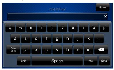
Use the keyboard to make the new entry. Touch **Cancel** to return to the "Ethernet Setup – Edit IP Table Entry" screen. Touch the "x" in the text field to clear any
