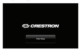
Tap the **Setup** button to display the TSW-752 **Setup** screen. The buttons on the **Setup** screen enable basic configuration prior to regular operation of the TSW-752.
