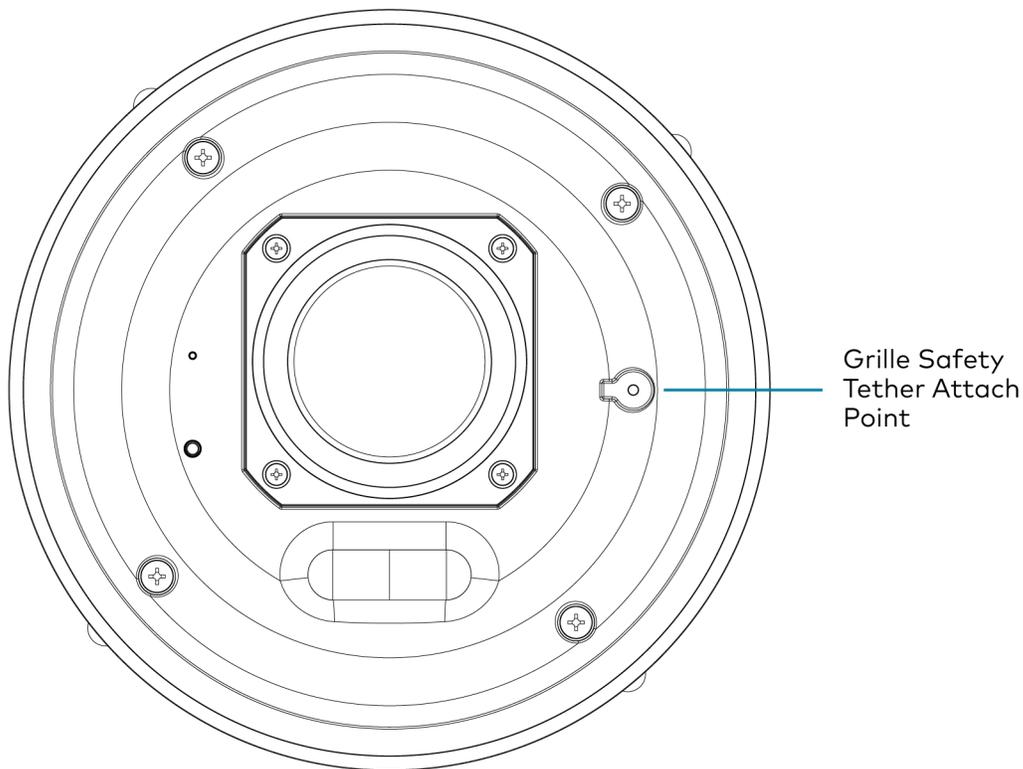
3. With the tether attached, place the grille in position on the speaker.
