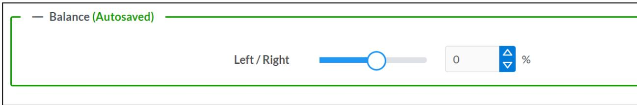
Balance values range from -50 to 50, adjustable in increments of 1. Positive values shift the balance to the right while negative values shift the balance to the left. To adjust the left/right balance of the stereo output signal, do one of the following:
