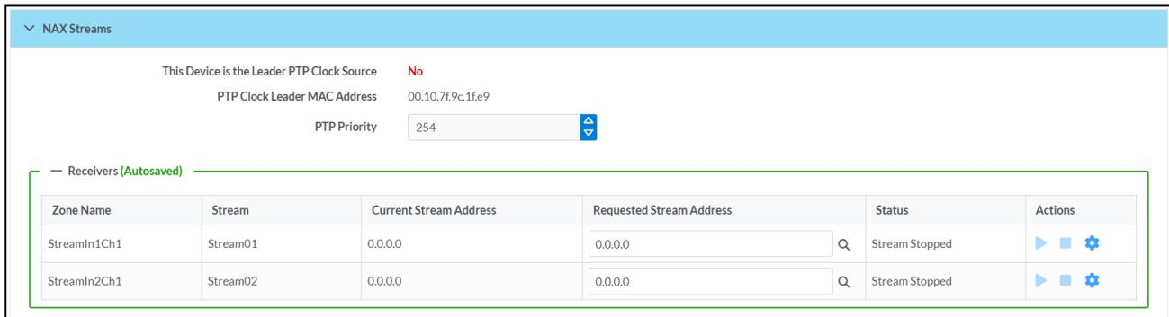
**Device is Leader PTP Clock Source** indicates whether the device is the leader for PTP on the network. **Yes** will be displayed in green when the local SAROS DM-NAX-IC4A-W is the PTP leader clock and **No** will be displayed in red when another PTP clock on the network is operating as the leader clock.
