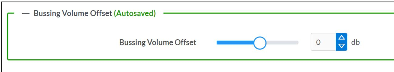
**Bussing Volume Offset** is an additional level compensation applied to the zone relative to any other zones it is grouped with via the **Bussing** feature.
