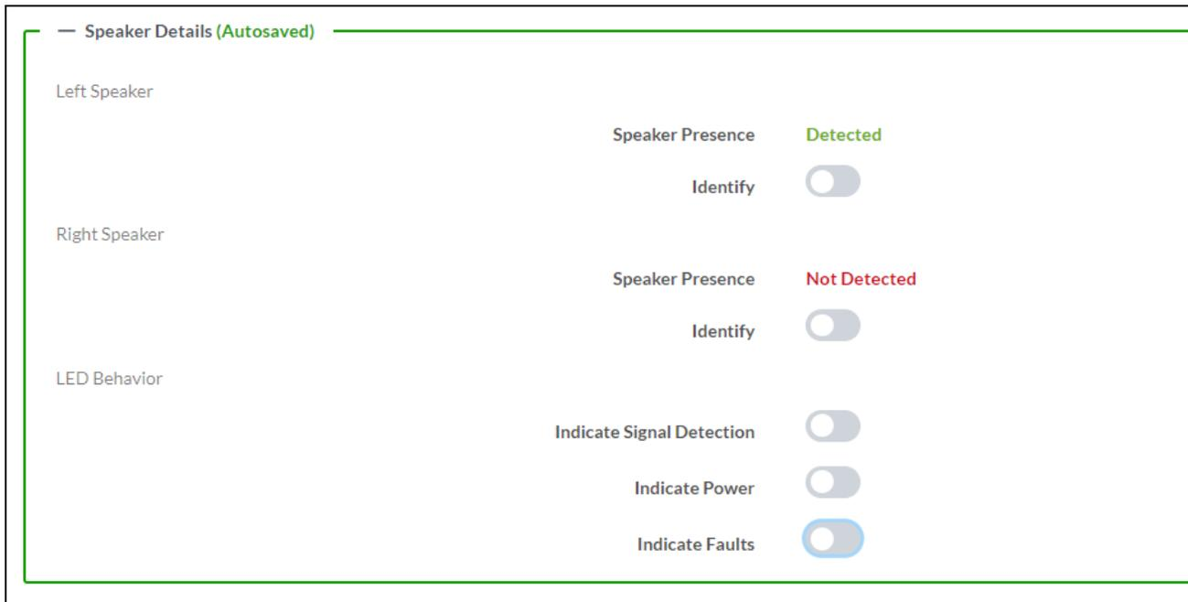
The **Speaker Presence** field for the **Left Speaker** will read **Detected** in green if the associated speaker is connected and detected by the SAROS DM-NAX-IC4A-W. It will read **Not Detected** in red if the associated speaker is not connected or detected. Set the **Identify** toggle to the right to cause the baffle LED of the associated speaker to blink. Set the **Identify** toggle to the left to stop the baffle LED from blinking.
