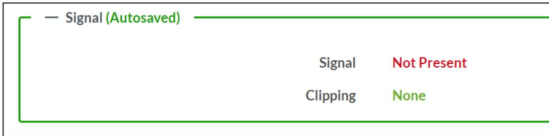
The **Signal** section is a read-only field that displays the **Signal** and **Clipping** status of the zone output.
