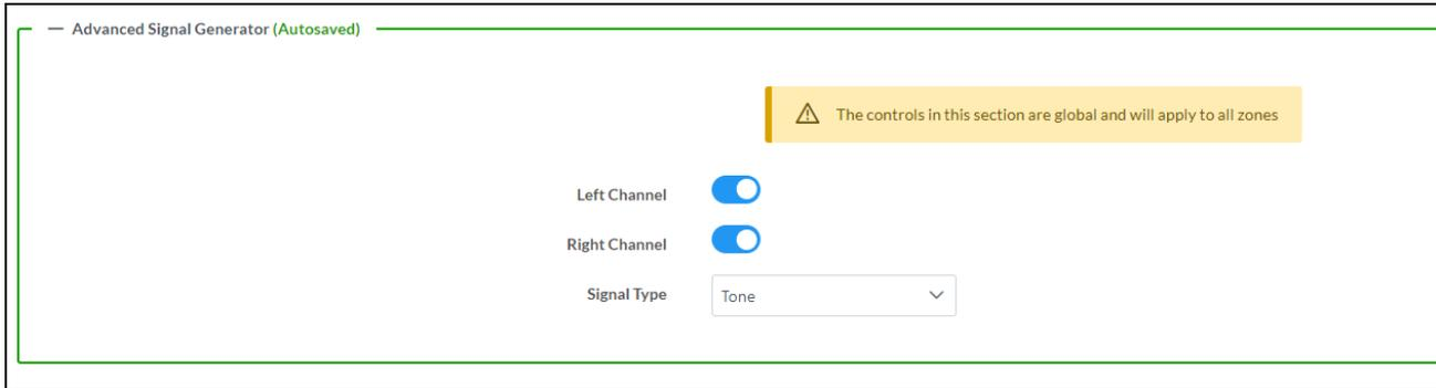
The advanced signal generator settings control the built-in signal generator directly, and are applied universally to all output zones of the device. The signal type for the generator can be set, and the left and right channels of the test signal can be individually enabled or disabled.
