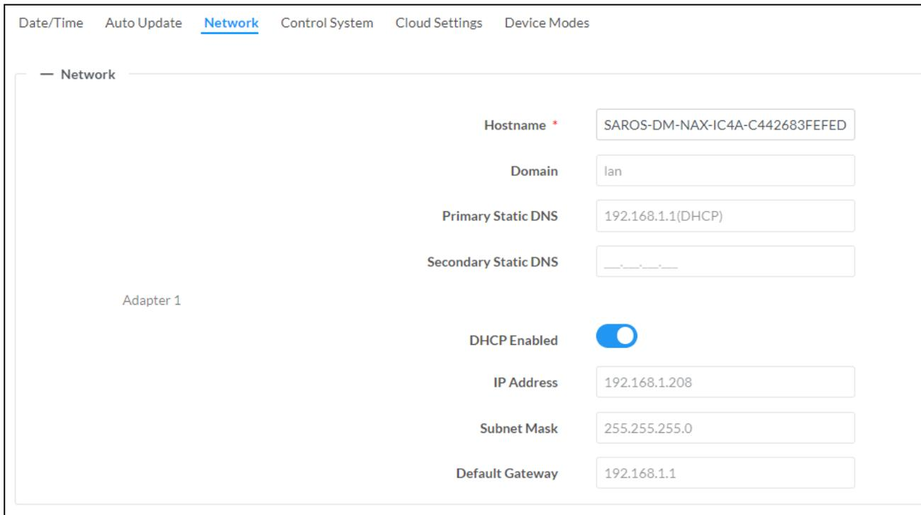
The screenshot shows the Network configuration page for the SAROS DM-NAX-IC4A-W. The page has a navigation bar with tabs for Date/Time, Auto Update, Network (selected), Control System, Cloud Settings, and Device Modes. The main content area is titled 'Network' and contains a subheading 'Adapter 1'. The settings are as follows:
