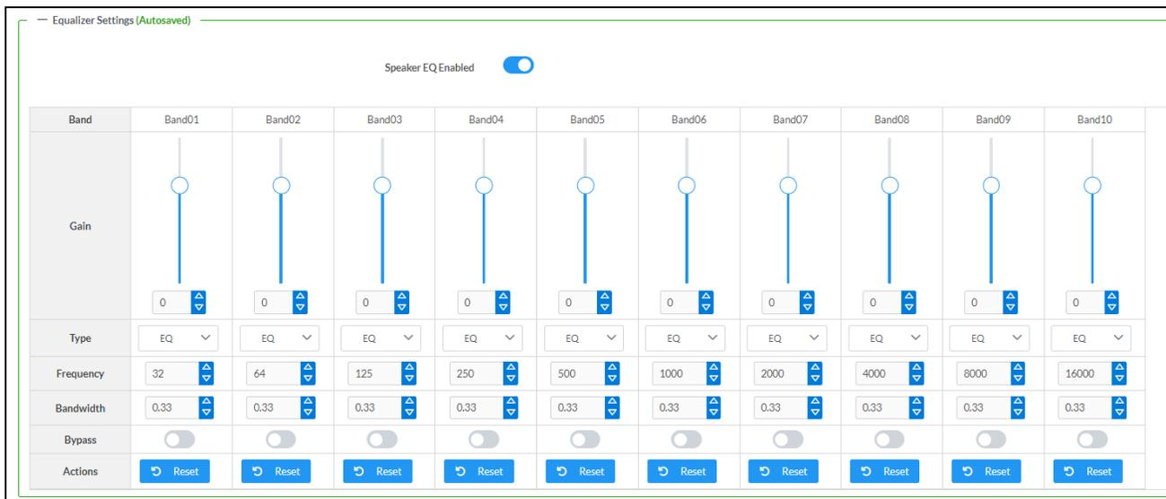
Each speaker output of the SAROS DM-NAX-IC4A-W has a dedicated ten-band equalizer that can be fully customized to tune the speaker output signal to the needs of an install. Each band can have a discrete gain, filter type, center frequency, and bandwidth set, and can also be bypassed. The equalizer itself can also be bypassed using the **Speaker EQ Enabled** toggle.
