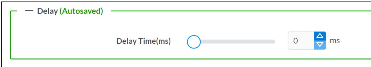
**Delay Time** values range from 0 ms to 85 ms, adjustable in increments of 1 ms. To set the delay, do one of the following:
