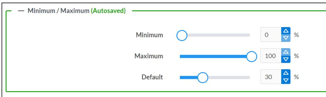
1. The minimum volume values range from 0 to 50%, adjustable in increments of 1%. To set the minimum volume of the zone, do one of the following:
