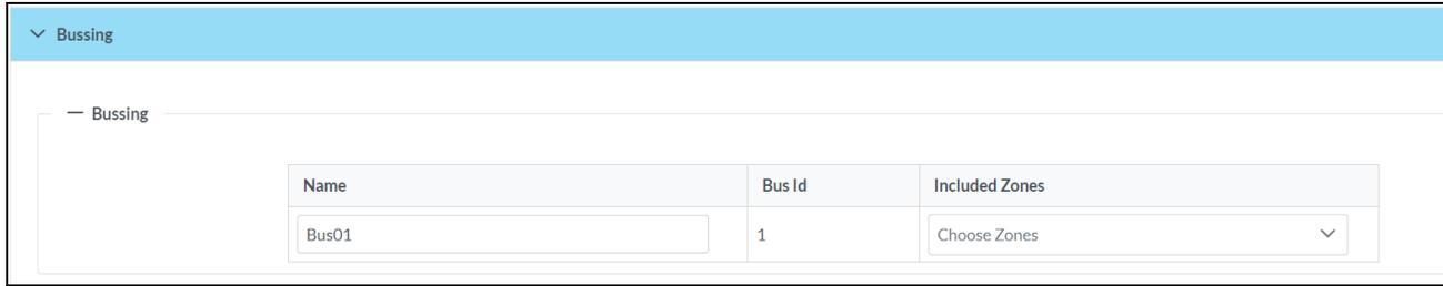
The **Bussing** feature on DM NAX devices allows an integrator to assign any number of selected zones to a fixed group of zones (bus). Zones in a bus track the other zones' volume and routing. For example, when the source or volume for one zone in the bus is adjusted, all other zones in that bus receive the same adjustment. You can create a single output bus on the SAROS DM-NAX-IC4A-W.
