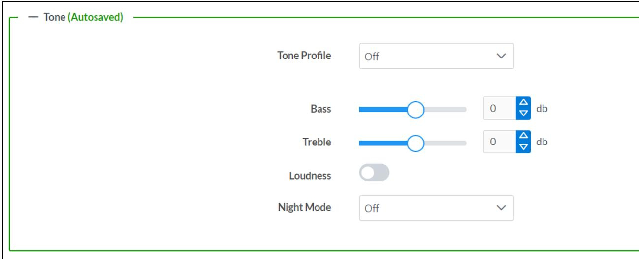
The **Tone** section provides adjustments for the **Tone Profile**, **Bass**, **Treble**, **Loudness**, and **Night Mode** settings of the zone output.
