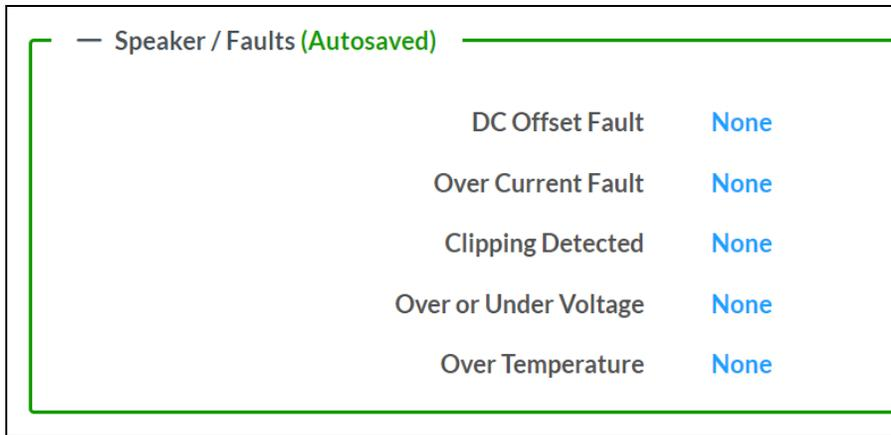
The **Speaker / Faults** section is a read-only field that displays the status of the **DC Offset Fault**, **Over Current Fault**, **Clipping Detected**, **Over or Under Voltage**, and **Over Temperature** detectors for the zone output. If clipping or a given fault type is detected, then its corresponding readout displays **Fault Detected** in red. Otherwise, it displays **None** in blue.
