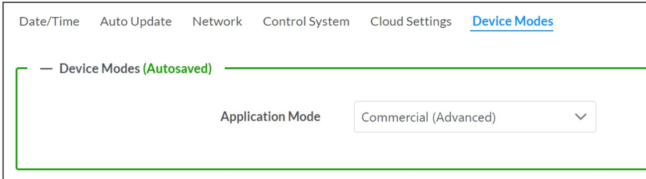
The **Application Mode** setting determines which options and controls are available in the rest of the **Settings** tab of the interface. To change the **Application Mode**:
