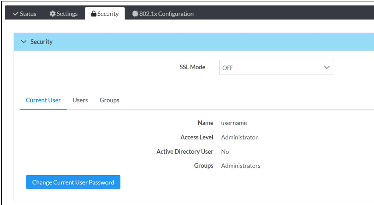
Select **Encrypt and Validate**, **Encrypt**, or **OFF** in the **SSL Mode** drop-down menu, to specify whether to use encryption. By default, **SSL Mode** is set to **OFF**.
