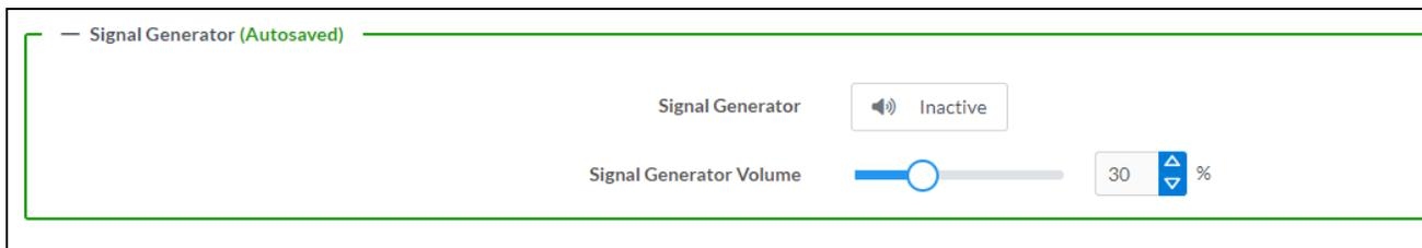
The SAROS DM-NAX-IC4A-W has a built-in signal generator that allows an integrator to send an audio signal to any number of selected zones to test output functionality.
