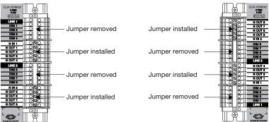
Wiring the Terminal Block to the Module (Right-Side Double-Wide Enclosures)
