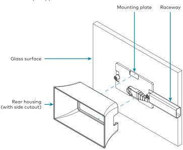
NOTE: The raceway shown in the image above conceals cables running to the touch screen and can be installed to the surface before or after the rear housing is installed. For more information, refer to the "Install the Raceway Kit" section.
