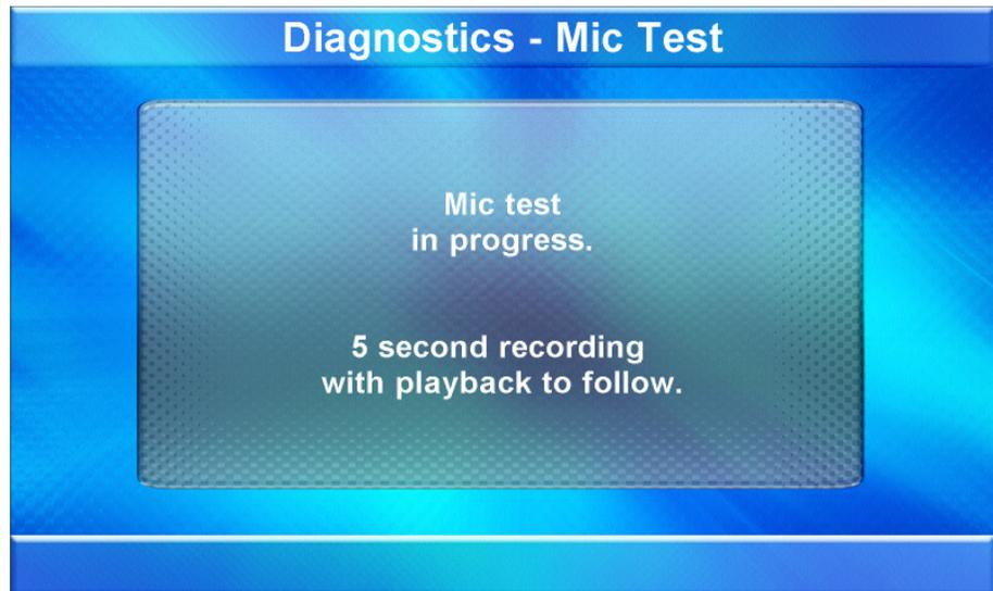
This screen performs a test of the TPMC-9’s built-in microphone. The touch screen records audio for five seconds and then plays back the recorded sound. Speak into the microphone on the front of the TPMC-9 and the recording is played back to confirm the microphone is functioning. When playback is finished, the display goes back to the “Diagnostics” menu.
