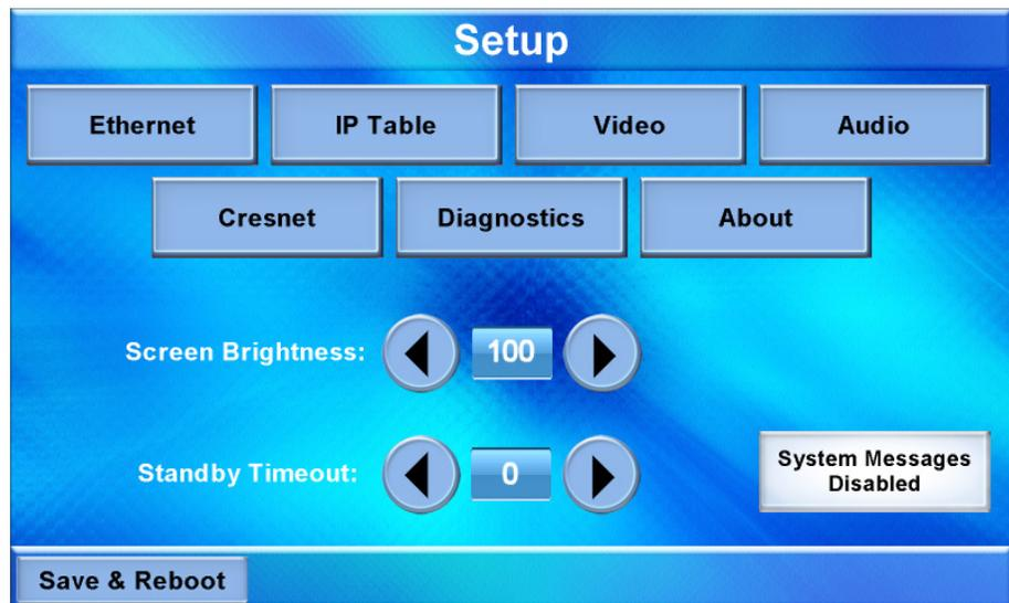
The “Setup” menu provides access to all basic functions and parameters. There are buttons for **Ethernet**, **IP Table**, **Video**, **Audio**, **Cresnet**, **Diagnostics** and **About**. There are also buttons to increase and decrease *Screen Brightness* and *Standby Timeout* as well as a button to enable/disable system messages and a **Save & Reboot** button to save settings and reboot the touch screen.
