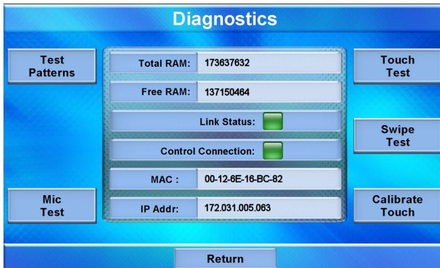
The “Diagnostics” menu contains buttons for **Test Patterns**, **Touch Test**, **Swipe Test**, **Mic Test** and **Calibrate Touch**. This screen also displays *Total RAM*, *Free RAM*, as well as the current MAC and IP addresses. A *Link Status* indicator lights in green to show Ethernet activity and a *Control Connection* indicator lights in green to show a control system connection.
