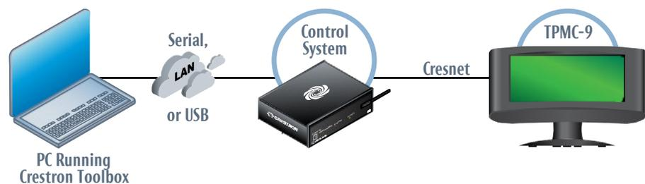
TPMC-9 connects to control system via Cresnet:
