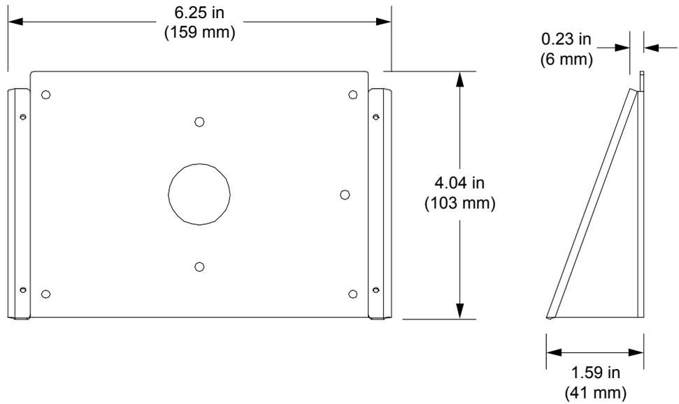
*Plastic Enclosure Overall Dimensions (Rear View)*
