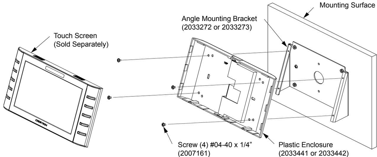
7. Secure the touch screen to the plastic enclosure with Phillip head screws. Alternatively, security Torx screws can be installed using a Torx screwdriver bit (both included with touch screen), as shown in illustration on page 8.
