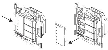
3. Press the new button assembly onto the device. It might be necessary to squeeze the sides of the button assembly to allow for easier button assembly installation.
