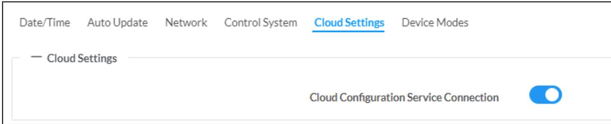
Set the **Cloud Settings** toggle to enabled (right) or disabled (left) to specify whether the DM-NAX-AUD-IO can communicate with the XiO Cloud® platform.
