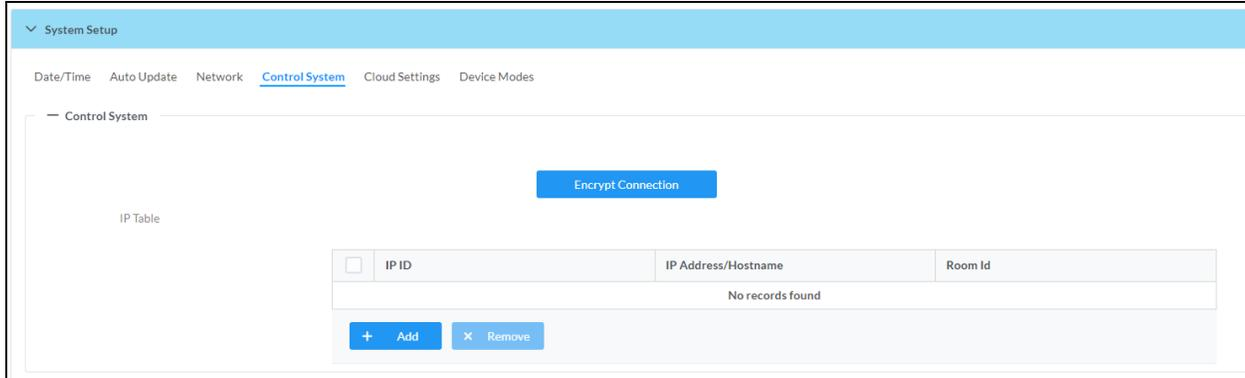
1. Select **Encrypt Connection** to navigate to the **Security** tab to configure encryption settings.
