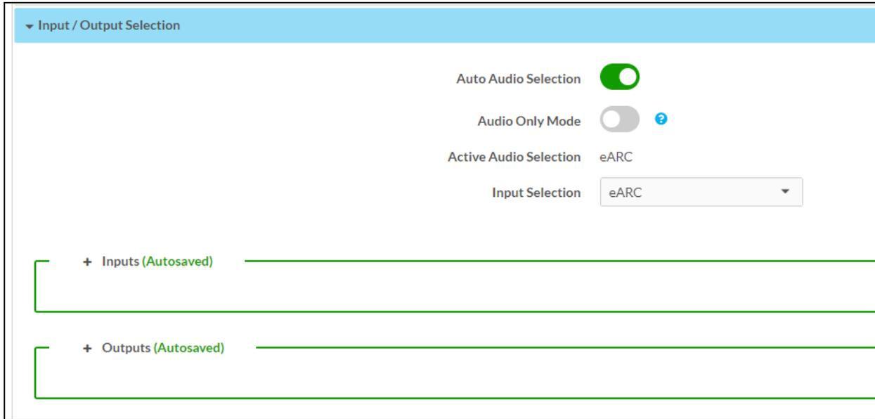
The **Auto Audio Selection** setting determines whether the active audio input of the DM-NAX-XSP is driven automatically by signal detection, or driven manually by either the **Input Selection** drop-down menu or programming.
