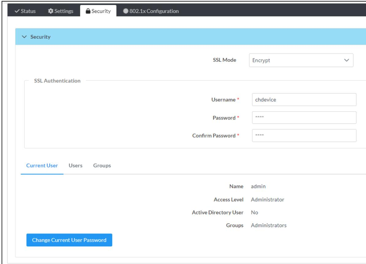
Select **Encrypt and Validate, Encrypt,** or **OFF** in the **SSL Mode** drop-down menu, to specify whether to use encryption. By default, SSL Mode is set to **OFF**.
