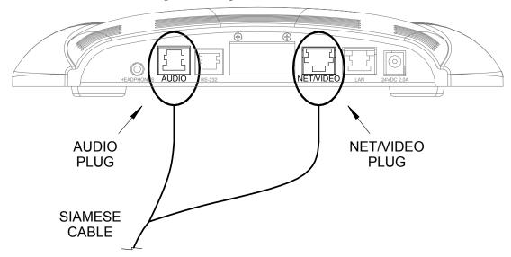
2. Refer to the diagram below. At the TPS-IMC (or optional TPS-IMW, not shown), attach the Siamese cable plug labeled **NET/VIDEO** to the **NET/VIDEO** port and the plug labeled **AUDIO** to the **AUDIO** port.
