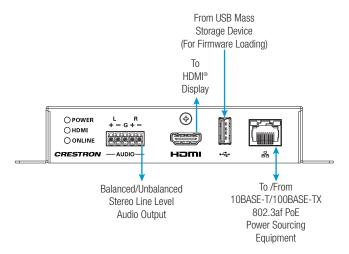
**NOTE:** The Ethernet port  $(\frac{\Box}{\Box})$  is a PoE (Power over Ethernet) PD (Powered Device) port.
