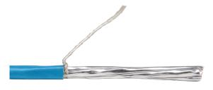
3. Remove the foil shield from each of the four twisted wire pairs, leaving 1/8 inch (3 mm) of the foil shields from the edge of the outer jacket.
