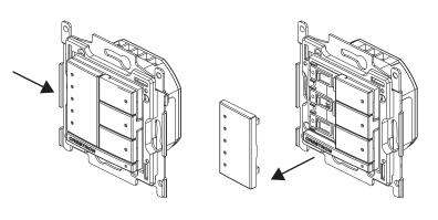
3. Insert the new button assemblies onto the device by pressing them into the device. It might be necessary to squeeze the sides of the button assembly to allow for
