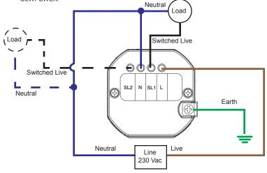
When making connections to the device insert the wires into the back of the unit.Use a small flat head screwdriver to tighten the connection.
