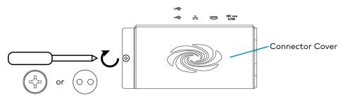
**NOTE:** For additional security, replace the screws with the included spanner screws. A 1/4 in. bit is supplied to install the spanner screws.
