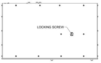
3. Using the Hex key, turn the locking screw counterclockwise to lock the drawer. To unlock the drawer, use the Hex key to turn the locking screw clockwise.
