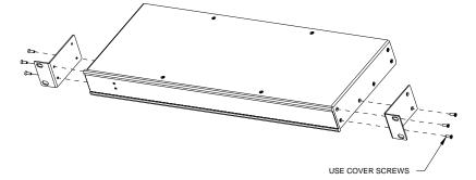
4. Repeat procedure (steps 1 through 3) to attach the remaining ear to the opposite side.
