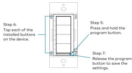
6. While holding the program button, press all of the buttons in the new layout. The LED next to the pressed button lights.
