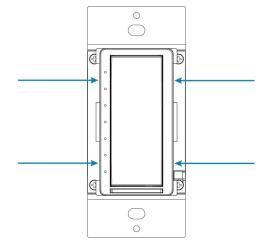
Squeeze at the arrow points and pull to remove the button assembly.
