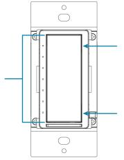
Press to turn on the load. Press and hold to raise the light level.
