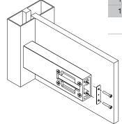
6. Connect the LAN cable to the touch screen. Then, attach the TSS-752 to the mullion mount by carefully positioning it over the four screws protruding from the front of the mullion mount. Slide the TSS-752 toward the mullion until the touch screen clicks into place.
