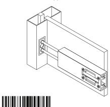
5. Use the included metal locking plate and the two included 08-32 x 5/8" screws to secure the mullion mount. (These screws require a #8 socket.)
