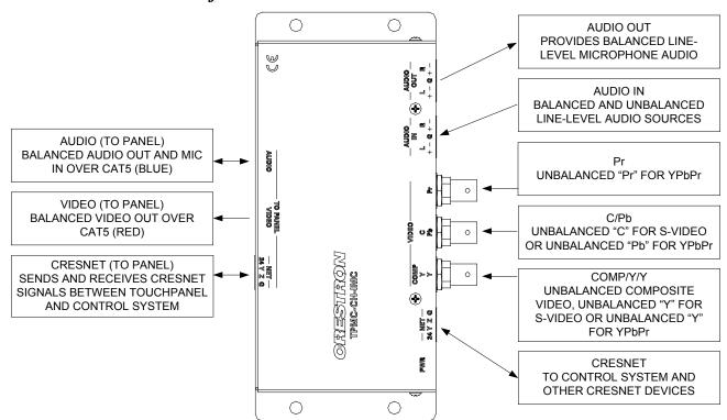
A triamese cable included with the touchpanel has an RJ-45 connector with a blue cover to match the blue label on the TPMC-CH-IMC and an RJ-45 connector with a red cover to match the red label on the TPMC-CH-IMC. The cable also has a 4-position mini terminal block connector for making a network connection between the touchpanel and the TPMC-CH-IMC.
