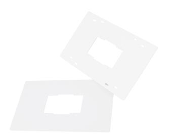
The Crestron® TSW-1070-RMB-3 is a retrofit mounting bracket that allows an older TPS-6L touch screen to be easily upgraded to a current generation TSW-1070 or TSS-1070 series touch screen. The TSW-1070-RMB-3 installs into an existing back box or wall cutout using the provided mounting hardware and without requiring any patching or tearing to the surface.
