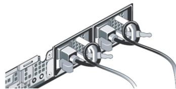
6. Plug the power cable(s) into suitably powered and grounded electrical supplies. An uninterruptable power supply (UPS) or power distribution unit is recommended.
