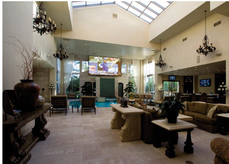
screen is down," Kermani explains. The atrium also includes a distributed audio system using a combination of ceiling and flush-mount loudspeakers and subwoofers, including waterproof speakers near the pool.
