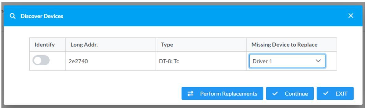
**TIP:** Set the **Identify** toggle to the right position in the replacement device's table row to turn it on and ensure it is the correct device. Set the **Identify** toggle to the left to turn that device off.
