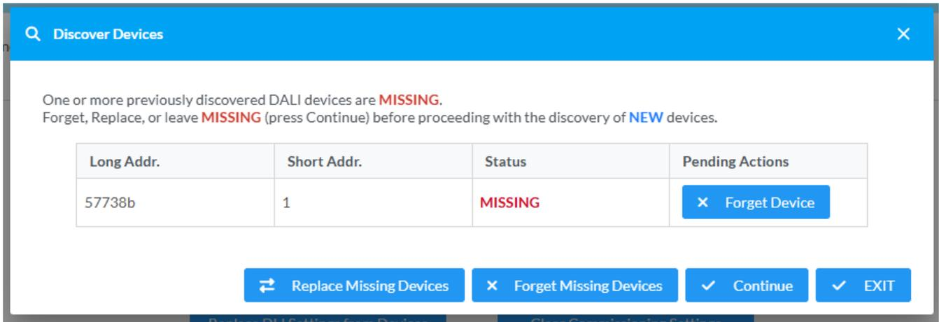
**NOTE:** **Replace Missing Devices** can only be selected if at least one new device was detected on the DALI loop with the same device type as any of the **MISSING** devices.
