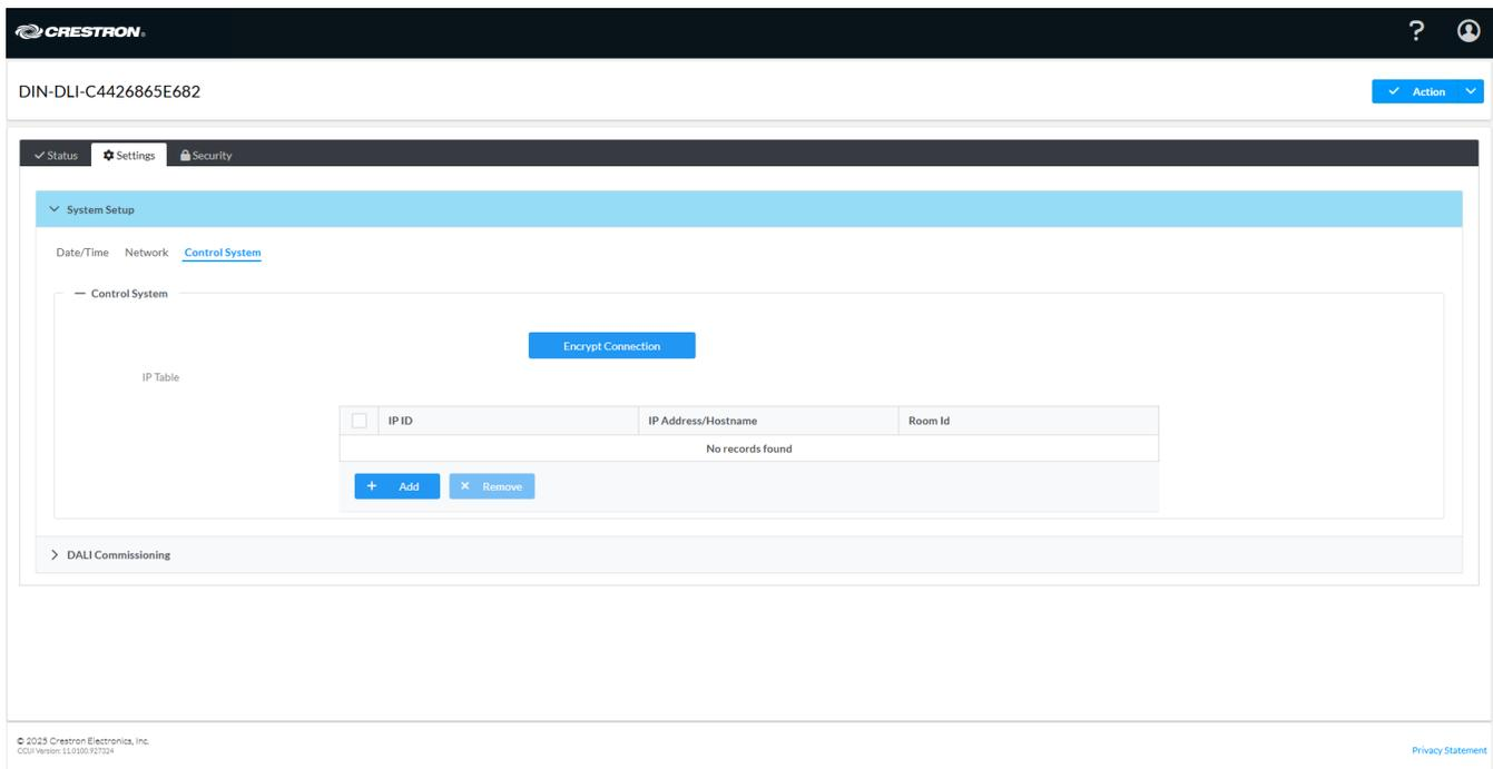
1. Select **Encrypt Connection** to navigate to the **Security** tab to configure encryption settings. Refer to [Security on page 45](#) for details.
