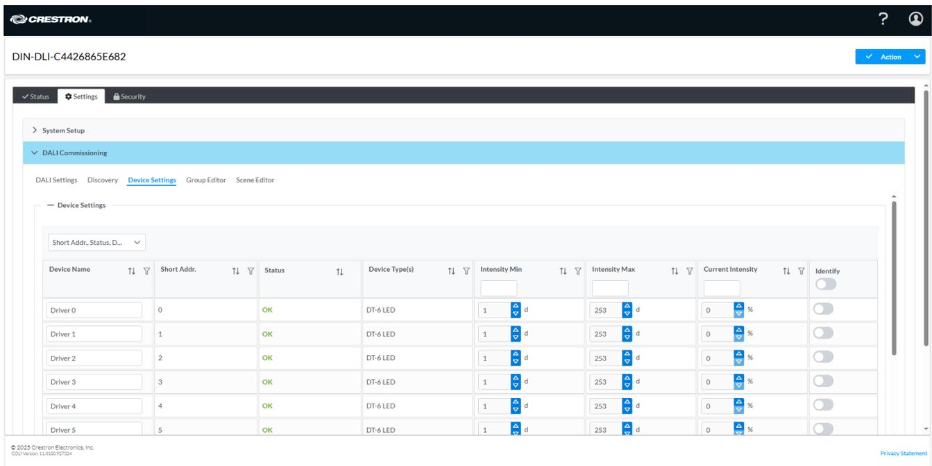
Each row in the **Device Settings** table represents a discovered DALI device that has been added to the DIN-DLI. Each column is tied to a DALI device setting or DALI device information readout.
