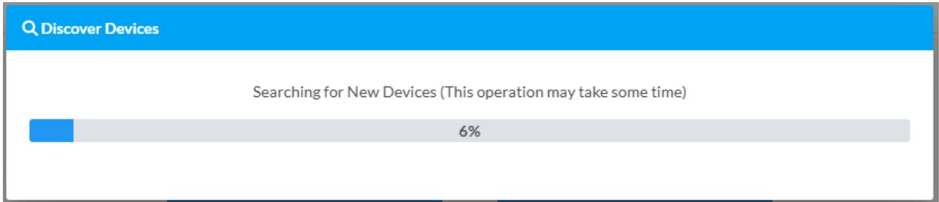
Once the discovery process completes, if any devices already added to the DIN-DLI were missing from the DALI loop, a **Discover Devices** table with just those missing devices will appear with options to either **Replace Missing Devices**, **Forget Missing Devices** (individually or all at once), **Continue**, or **EXIT**.
