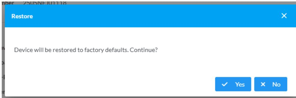
2. Select **Yes** to restore the device to factory default settings. Select **No** to cancel the restore operation. When **Yes** is selected, the **Restore** status message box appears. Wait for the device restore to complete before attempting to reconnect to the web interface.
