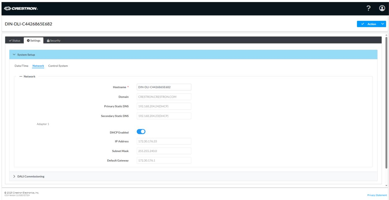
Enter a custom hostname in the **Hostname** field. By default, the hostname of the device consists of the model name followed by its MAC address. For example, DIN-DLI-C4426865E682.
