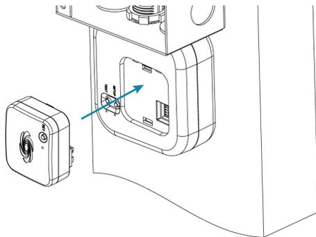
If the J-box module needs to be removed, place your thumb on the side of the J-box module that is closest to the J-box and gently push the module away from the J-box. The module should easily separate from the J-box device.
