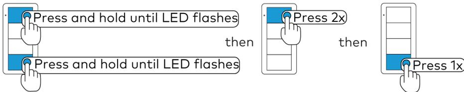
**NOTE:** Scene Setting mode exits after 5 minutes when initiated from an ac-powered keypad or 1 minute when initiated from a battery-powered keypad.
