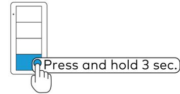
3. Press the bottom button of the keypad to cycle through all of the load controllers in the Zūm space until the desired load starts flashing.
