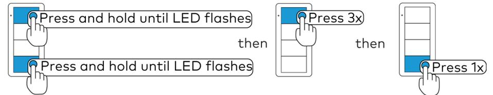
**NOTE:** Use the keypad that has been selected for controlling the load to perform the entire remote linking process.
