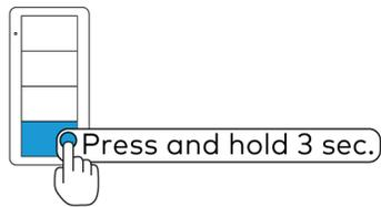
3. Press the bottom button of the keypad repeatedly to cycle through all of the load controllers in the Zūm space until the desired load starts flashing.
