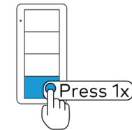
4. Adjust the light levels by holding the top button on the keypad to raise the light level or holding the bottom button on the keypad to lower the light level.
