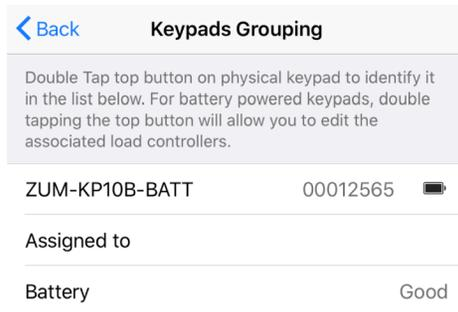
3. Double tap the top button on the keypad you wish to bind to a load. The keypad's menu appears in the Zūm configuration app. All devices in the Zūm room are listed.
