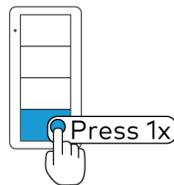
4. Press the top button of the keypad to assign the load controller as bound or not bound to the keypad. The LED on the keypad flashes to indicate that the load is bound or unbound.
