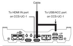
**NOTE:** Do not connect the HDMI connector to the HDMI OUT port on the CCS-UC-1. The cable is directional and cannot be used in that direction.
