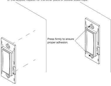
3. Ensure that the keypad is vertical, and press it against the wall. Press firmly to ensure that the keypad is properly secured to the wall.
