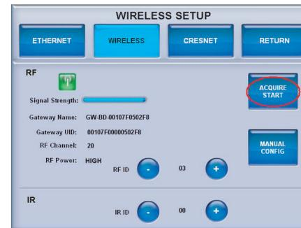
Before a TPS-6X can be used on a wireless network, it must first be acquired by a CEN-HPRFGW gateway (sold separately).
