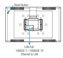
Carefully hold the touch screen over the mounting bracket and gently place it in position.The magnets on the rear of the touch screen hold it in place on the mounting bracket.
