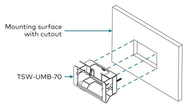
6. Reach into the assembly and push the rear half back so that it is behind the mounting surface completely. Ensure the front of the assembly is level.
