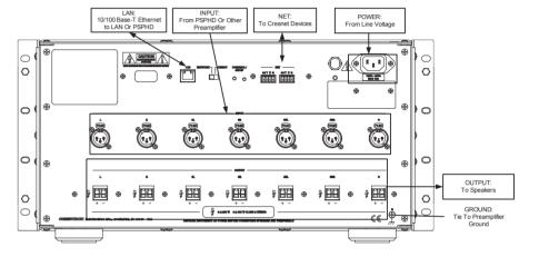
To connect the PROAMP-7X250 to a PSPHD, refer to the diagram below for additional connection information
