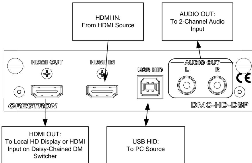
**NOTE:** The **AUDIO OUT** port contains a 2-channel downmix of the audio portion of the HDMI input signal.
