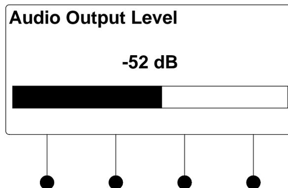
2. Turn the selection knob to adjust the audio output level.
