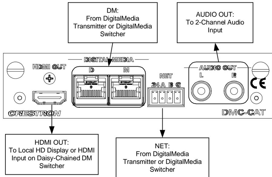
**DMC-CAT-DSP DM CAT Input Card with Down-mixing for DM Switchers**
