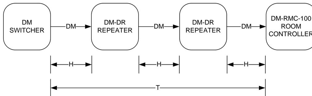
H = The maximum hop distance between a DM Switcher/ DM-RMC-100 Room Controller and a DM-DR Repeater
