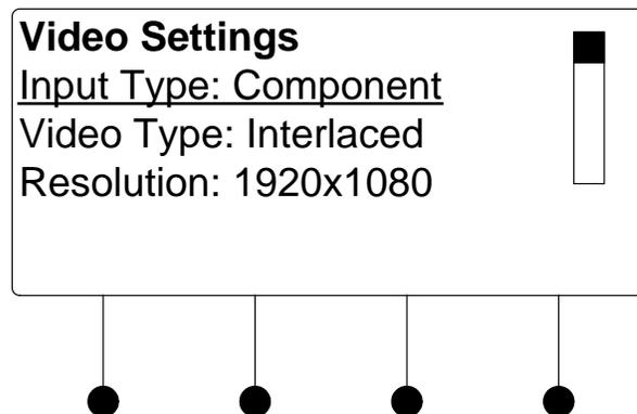
2. Turn the selection knob to view information on input type, video type, resolution, frame rate, and aspect ratio.
