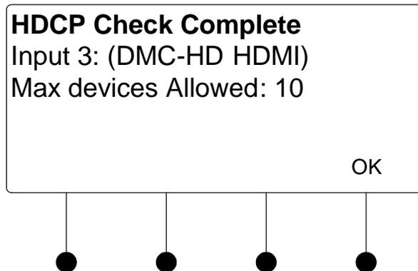
If the number of displays in use exceeds the number of devices supported by the source, an error message will be displayed.
