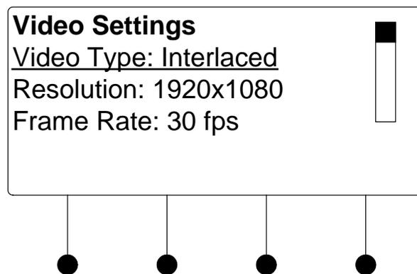
2. Turn the selection knob to view information on input type, video type, resolution, frame rate, and aspect ratio.
