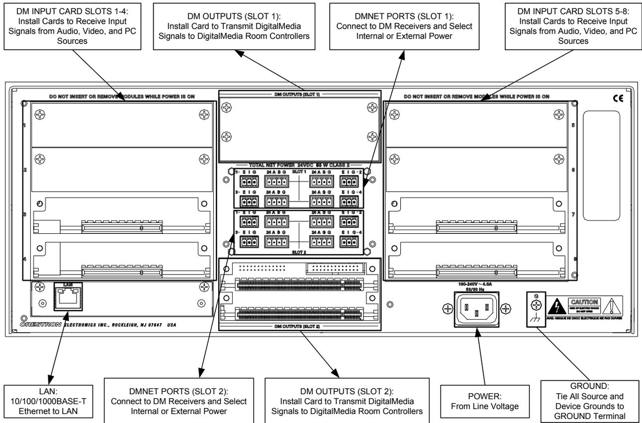
*Hardware Connections for the DM-MD16X16 Rear*
