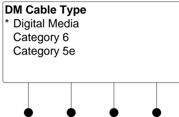
2. To select a different cable type, turn the selection knob to highlight the cable type to be used and press the **ENTER** button. An asterisk will appear next to the selected cable type.
