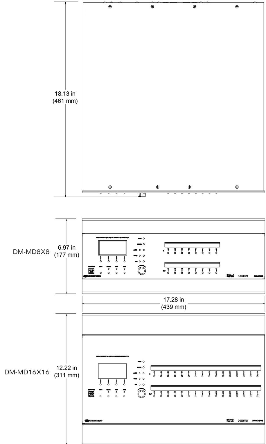
**NOTE:** Cable connections can extend the overall depth of the DM switcher by approximately two to three inches.
