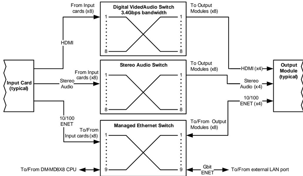
*Internal Block Diagram of the DM-MD16X16*
