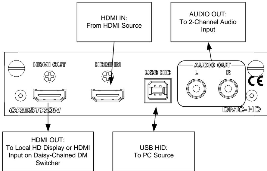
**NOTE:** Audio is present on the **AUDIO OUT** port when 2-channel audio is present on the HDMI input signal.
