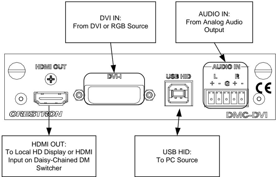
Balanced/unbalanced audio inputs are provided, utilizing five-pin terminal block connectors. For connection details, refer to the following table and diagrams.
