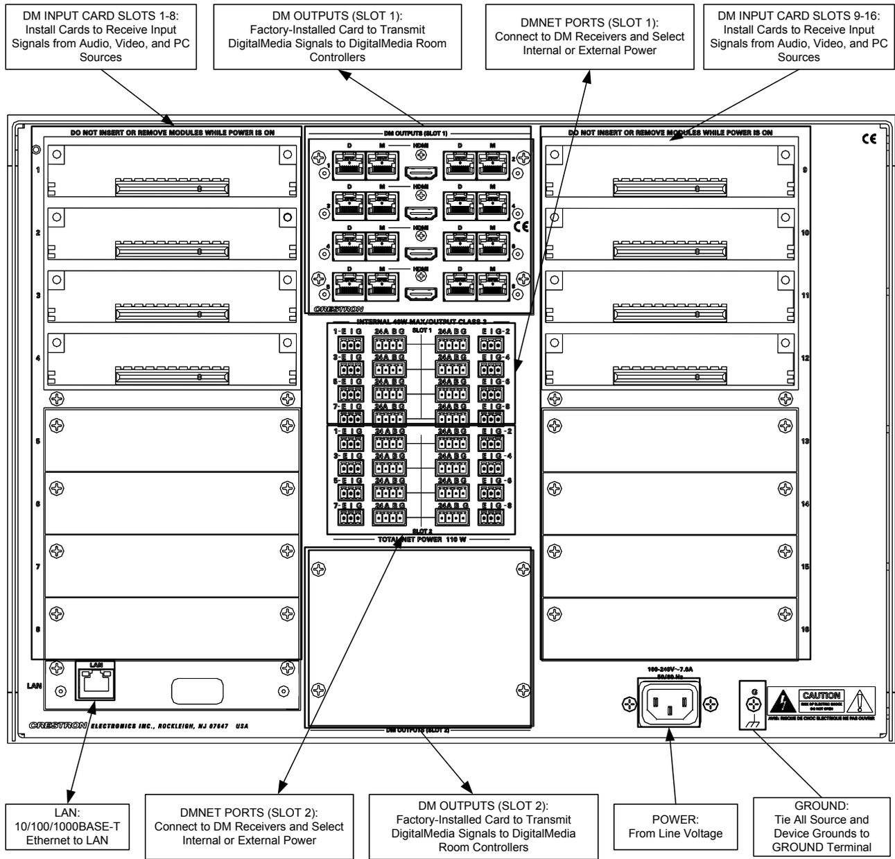
*Hardware Connections for the DM-MD32X32Rear*
