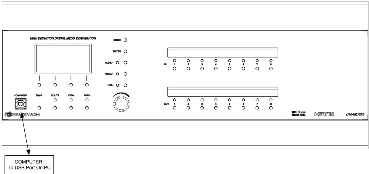
*Hardware Connections for the DM-MD16X16, Front*
