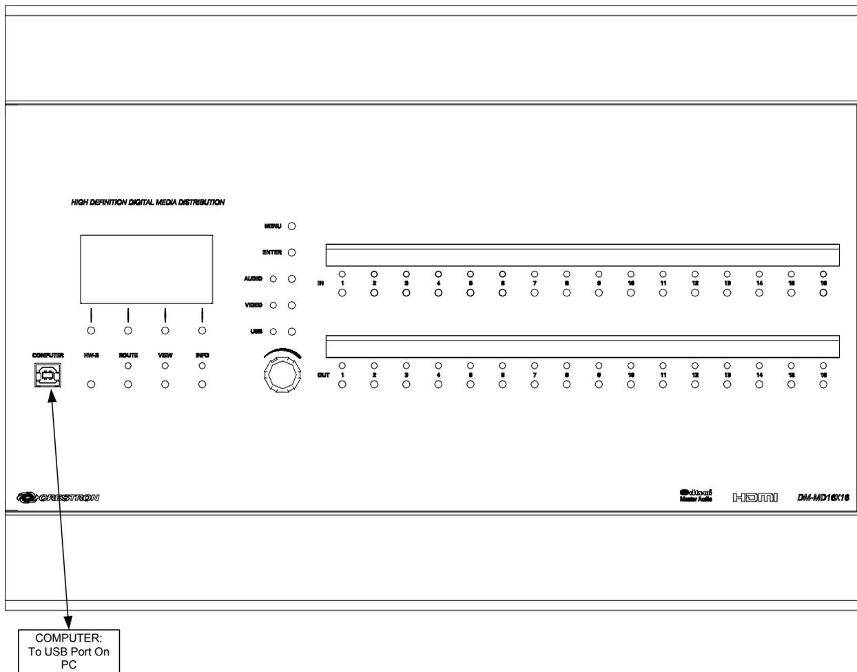
*Hardware Connections for the DM-MD32X32, Front*
