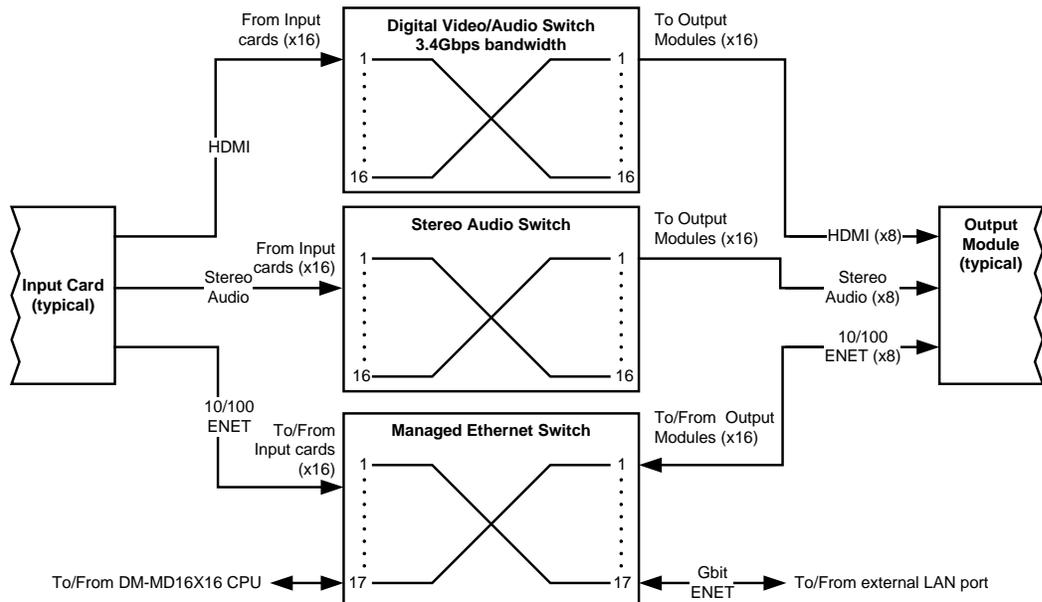
*Internal Block Diagram of the DM-MD32X32*
