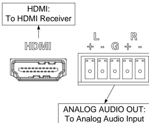
**NOTE:** The analog audio output will only function if it receives a stereo audio signal from a stereo source or a stereo downmix from a “-DSP” input card.
