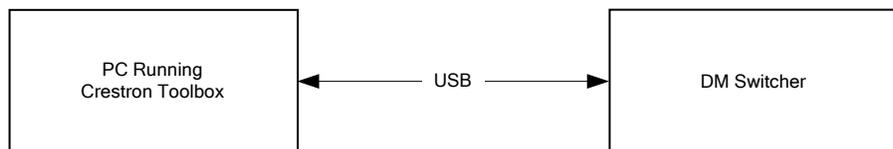
The **COMPUTER** port on the DM switcher connects to the USB port on the PC via the included Type A to Type B USB cable.
