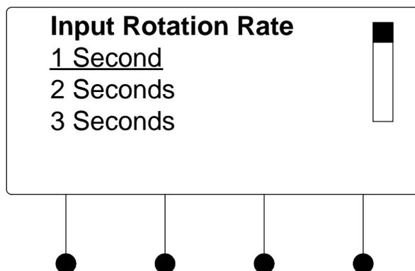
2. Turn the selection knob to highlight a rotate rate and press the **ENTER** button. Rotate rates from one to 60 seconds can be selected. The current selection is indicated with an asterisk (\*).
