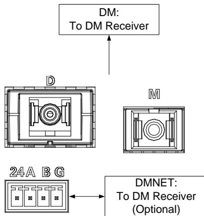
**NOTE:** When wiring the **24ABG** port, connect the **24** and **G** lines only. Do not connect the **A** and **B** lines.
