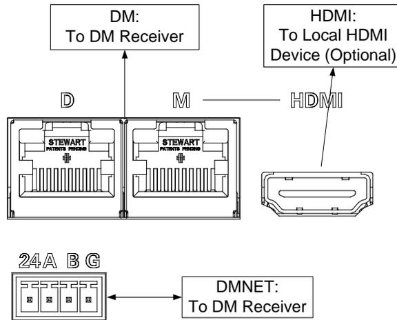
**NOTE:** The **DM** and **HDMI** ports can be connected simultaneously or individually.
