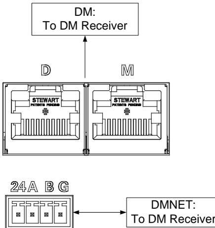
**D & M Ports Using DM Cable (with Optional HDMI Output)**
