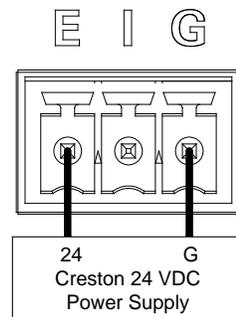
To power a DMNet port using the DM switcher’s internal power supply, install a jumper on the **EIG** connector from the **E** (External) pin to the **I** (Internal) pin as shown in the following diagram.
