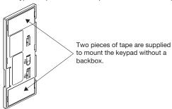
Ensure that the keypad is vertical and press it firmly against the wall to ensure it is properly secured.
