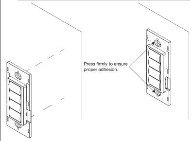
4. Remove the battery tab to turn on the keypad.
